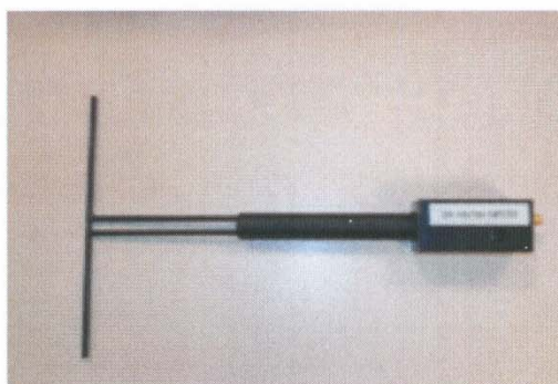
Figure 1 – Satimo COMOSAR Validation Dipole
