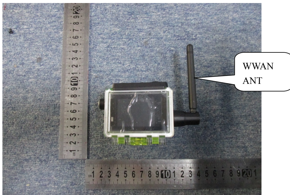
Fig. 3 Position of the antennas
