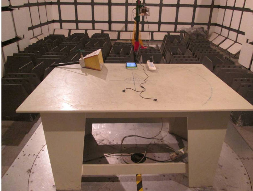
Radiated Emissions –Front View (Above 1GHz)
