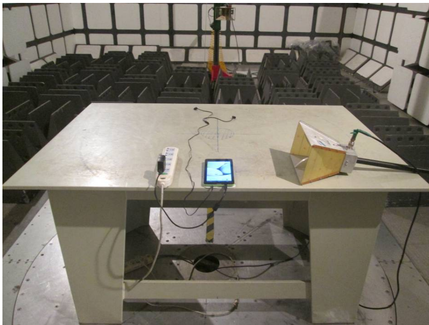
Radiated Emissions –Rear View (Above 1GHz)
