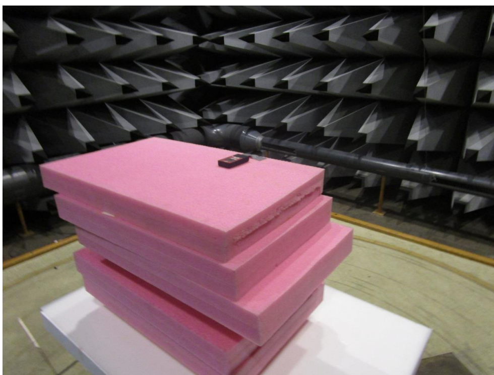
Photo 4.1.2 Test setup regarding measurement of radiated emission.
