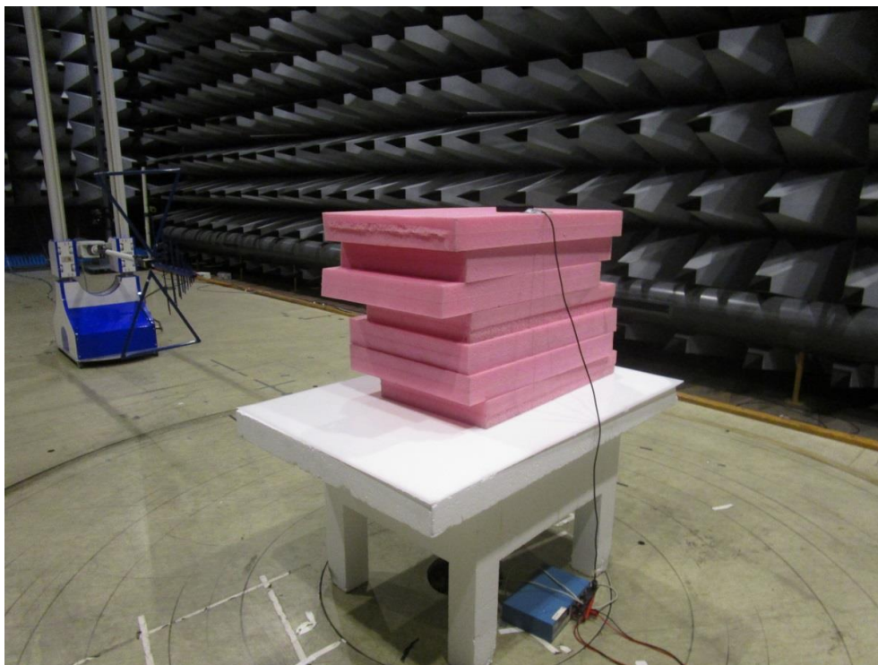
Photo 4.1.1 Test setup regarding measurement of radiated emission.
