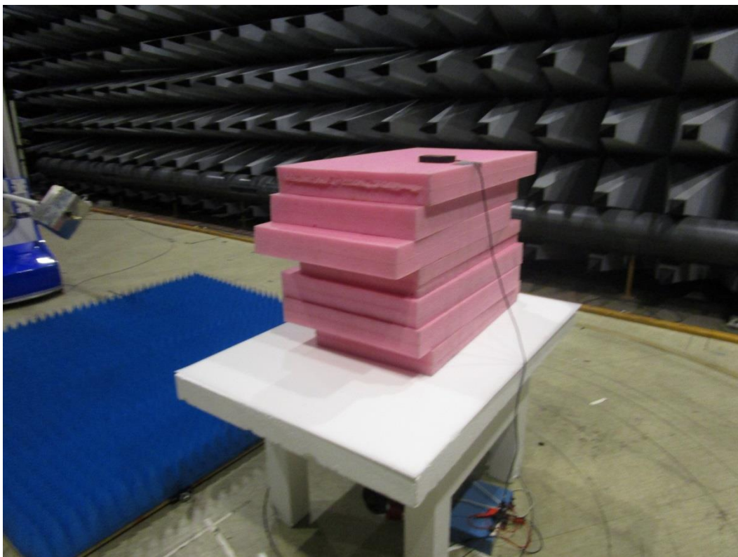
Photo 4.1.4 Test setup regarding measurement of radiated emission.
