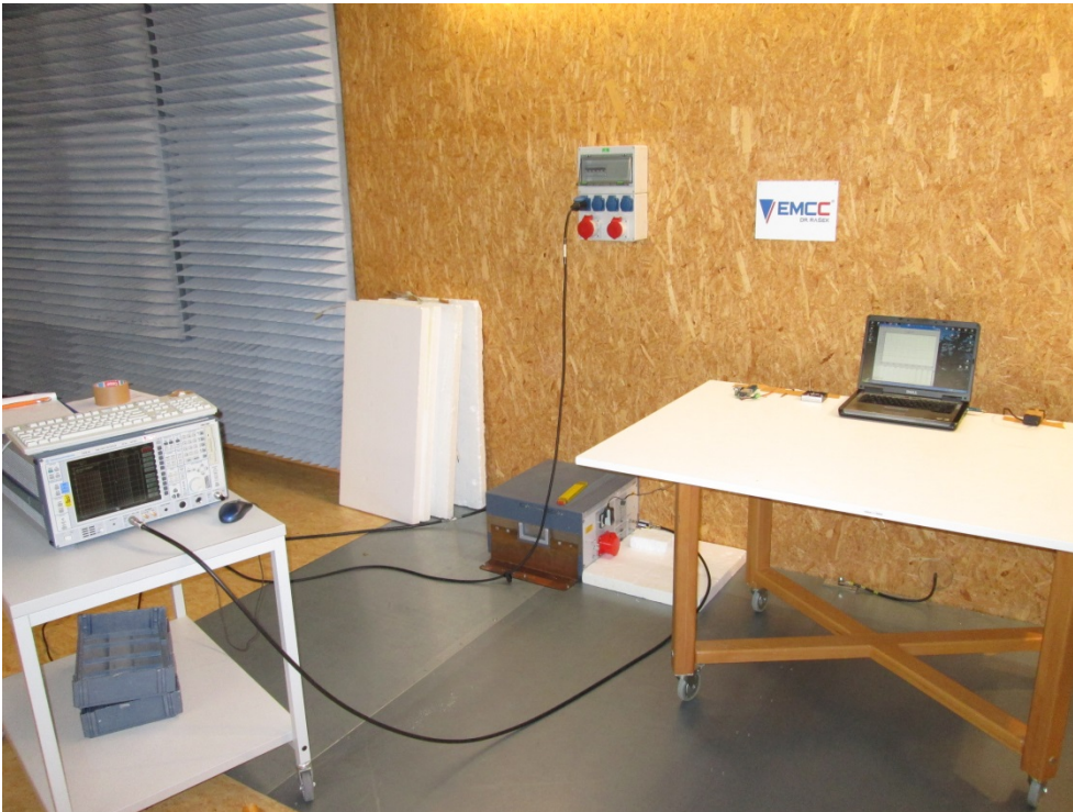
Photo A1-1: Conducted emissions measurement
