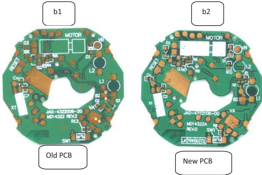
3, For this time modified, only the MCU and PCB layout change, No any other changes occur ; The LCD display、BLE Module、Product function are same . RF performance , parameter are same , no any RF change occur.
