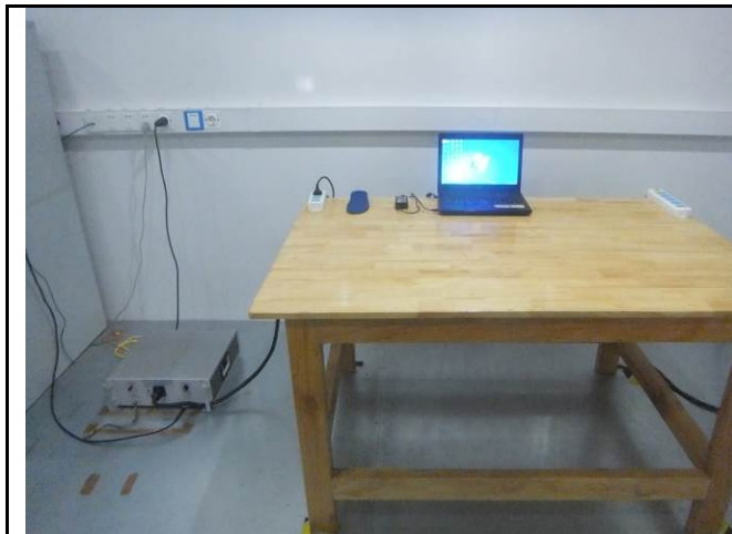
Conducted Emissions Test Setup – Front View
