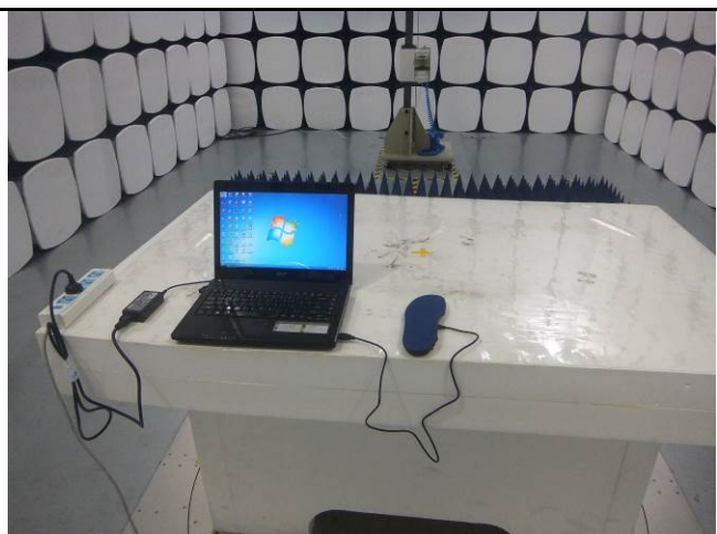
Radiated Spurious Emissions Test Setup Above 1GHz
