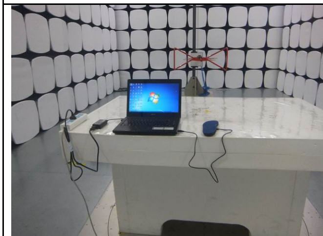
Conducted Emissions Test Setup – Front View
