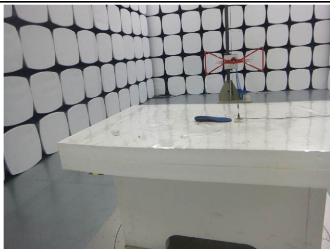
Radiated Spurious Emissions Test Setup Below 1GHz
