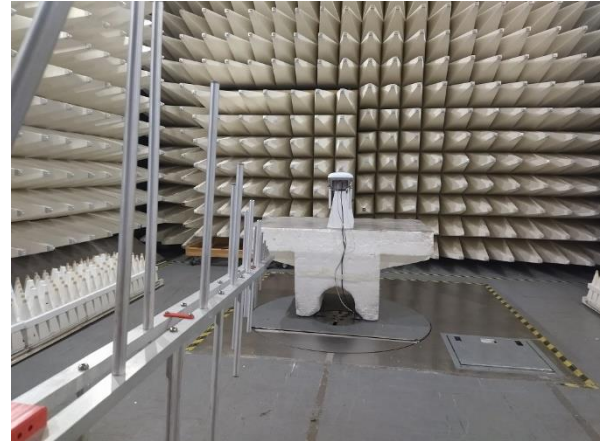
Photograph 7.1.1 Setup for spurious emission field strength measurements below 1000 MHz
