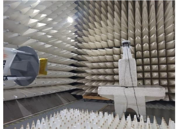
Photograph 7.1.2 Setup for spurious emission field strength measurements above 1000 MHz
