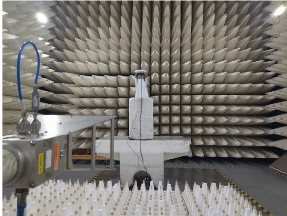
Photograph 7.1.2 Setup for spurious emission field strength measurements above 1000 MHz
