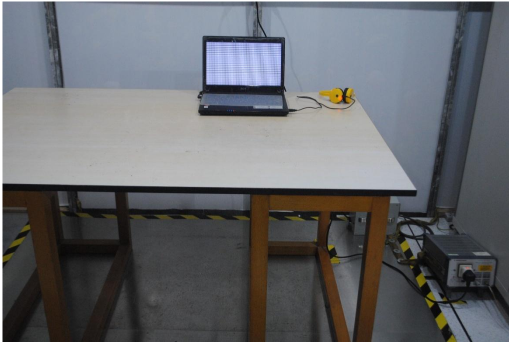
Conducted Emission test view
