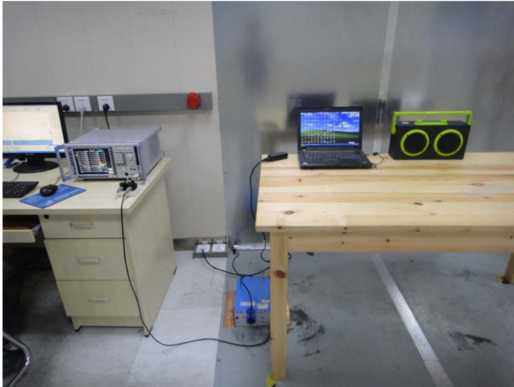
FCC RADIATED EMISSION TEST SETUP
