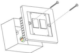
Match screw positions on the Switch Panel to the fixing holes of concealed metal box. Insert a 3" screw (provided in the box) and tighten using screw-driver.
