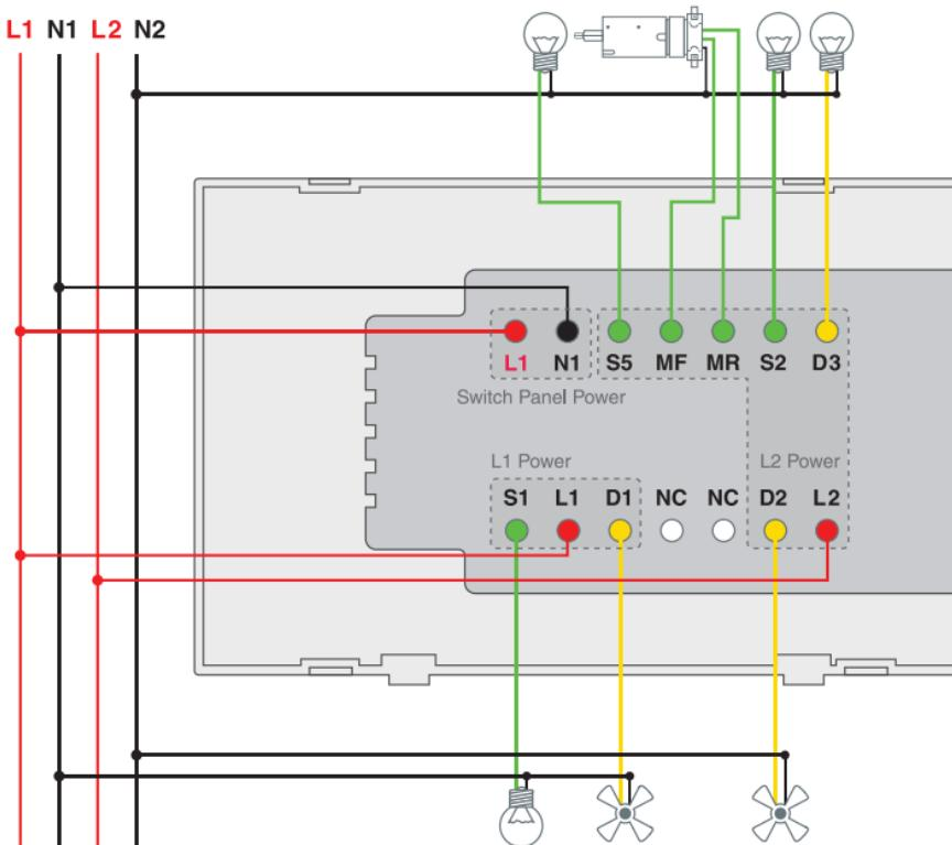
**Figure 3 - 6 Gang Switch Panel - Wiring Diagram**
