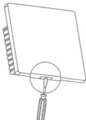
Un-box your Switch Panel and insert a flat screw-driver into one of the notches marked by the circle and twist slightly. Do this for rest of the notches to detach top-glass fixture from casing.
