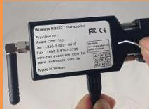
The Tx/ Rx LED light flashing 3 times, it finished one to one mode
