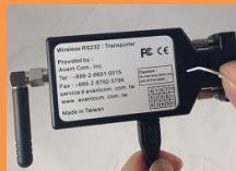
The Tx/ Rx LED light will be flashing 3 times, it finished the pairing.
