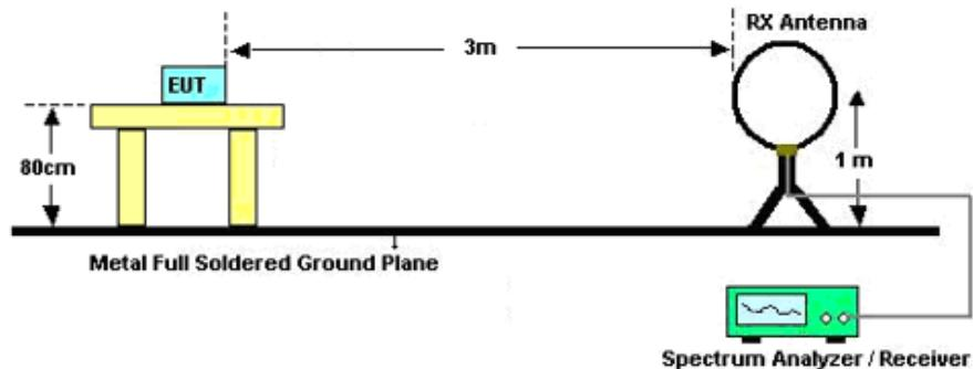
For radiated emissions from 30MHz to 1GHz
