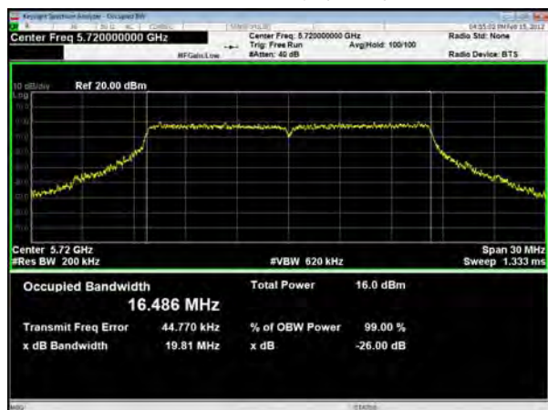
U-NII-2C, 802.11n HT40 Carrier frequency (MHz): 5510
