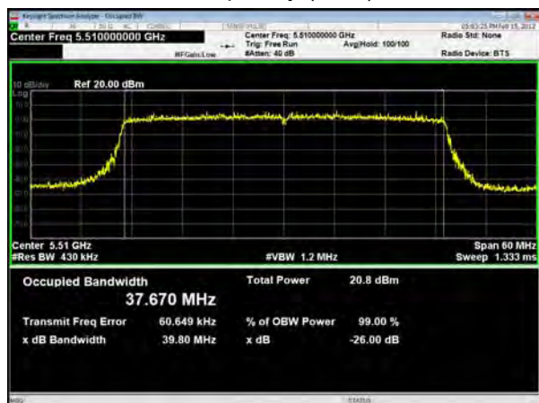
U-NII-2C, 802.11n HT40 Carrier frequency (MHz): 5550
