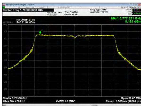
U-NII-3, 802.11ac VHT20, Channel No.: 165
