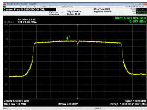
U-NII-2C, 802.11ac VHT160, Channel No.: 114
