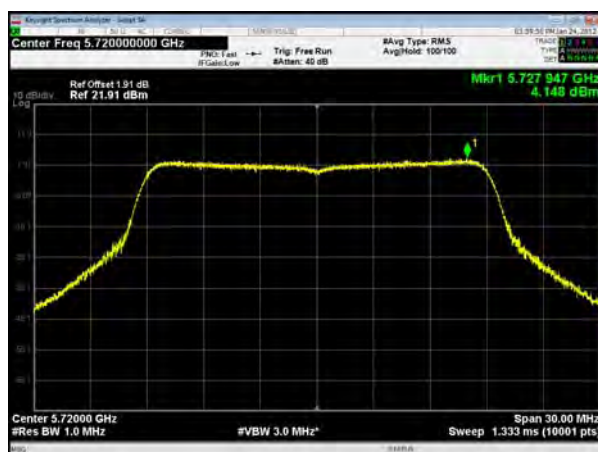
U-NII-2C, 802.11ac VHT80, Channel No.: 106
