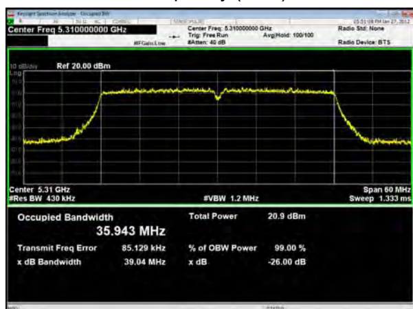
U-NII-2A, 802.11n HT40 Carrier frequency (MHz): 5310
