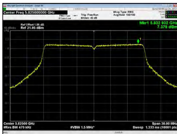
U-NII-3, 802.11ac VHT20, Channel No.: 165
