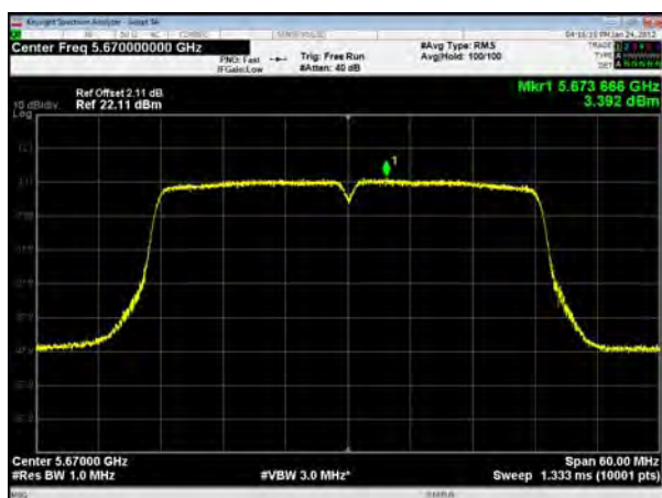
U-NII-2C, 802.11ac VHT40, Channel No.: 142
