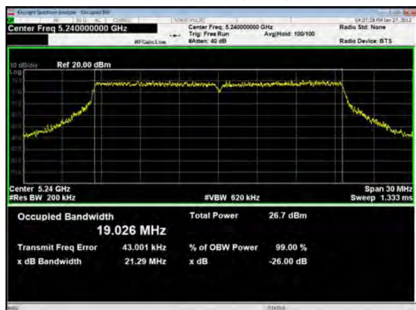
U-NII-2A, 802.11a Carrier frequency (MHz): 5260
