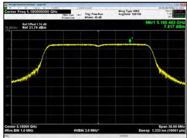
U-NII-1, 802.11ac VHT20, Channel No.: 40
