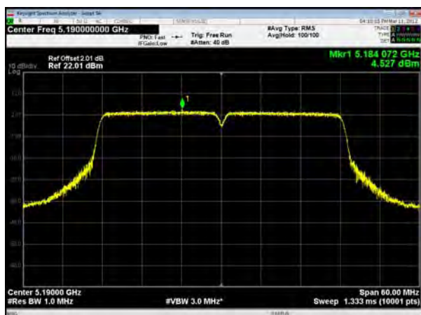
U-NII-1, 802.11ac VHT40, Channel No.: 38
