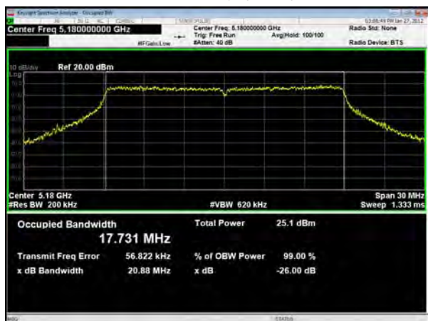
U-NII-1, 802.11n HT20 Carrier frequency (MHz): 5200
