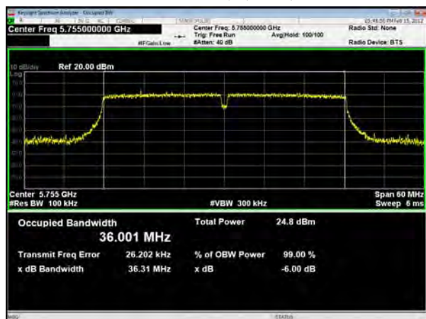
U-NII-3, 802.11n HT40 Carrier frequency (MHz): 5795
