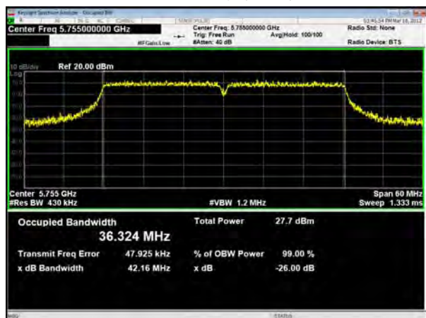
U-NII-3, 802.11n HT40 Carrier frequency (MHz): 5795
