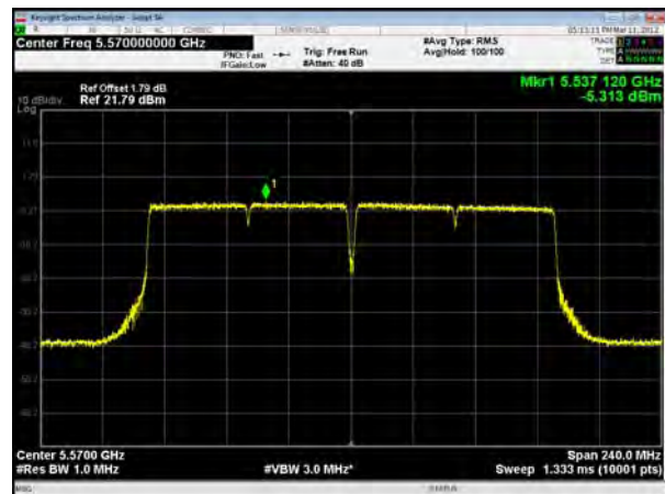
U-NII-2C, 802.11ac VHT160, Channel No.: 114
