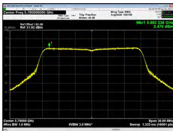
U-NII-2C, 802.11ac VHT20, Channel No.: 144
