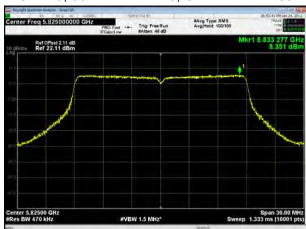
U-NII-3, 802.11ac VHT40, Channel No.: 151
