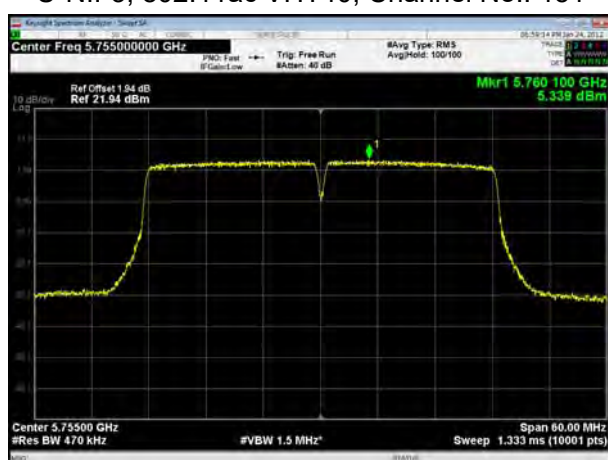
U-NII-3, 802.11ac VHT40, Channel No.: 159
