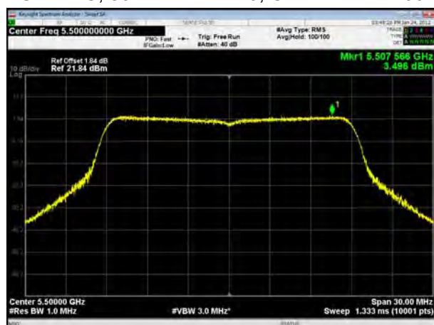
U-NII-2C, 802.11ac VHT20, Channel No.: 120
