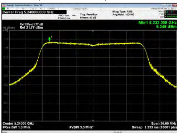
U-NII-1, 802.11ac VHT40, Channel No.: 38
