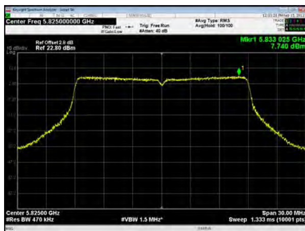
U-NII-3, 802.11ac VHT20, Channel No.: 165
