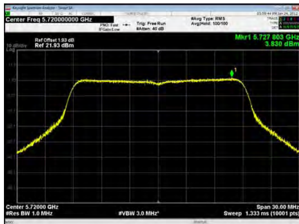
U-NII-2C, 802.11ac VHT40, Channel No.: 102
