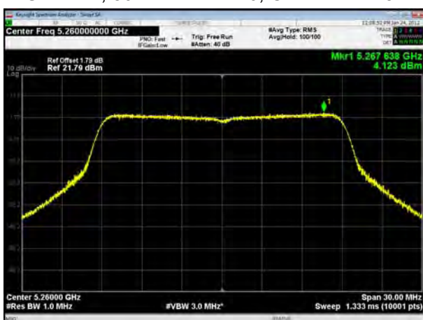
U-NII-2A, 802.11ac VHT20, Channel No.: 60
