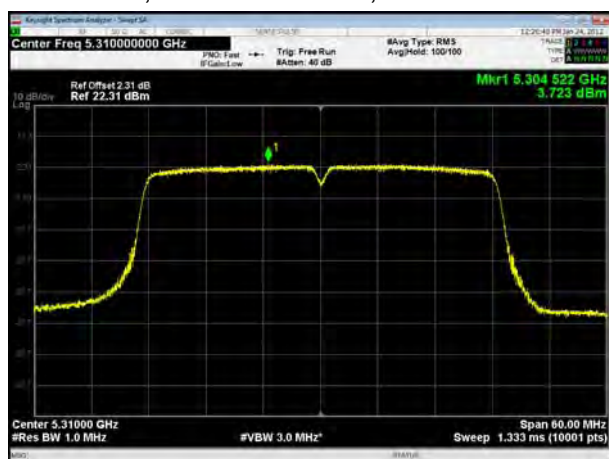
U-NII-2A, 802.11ac VHT40, Channel No.: 62
