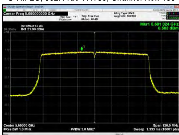
U-NII-2C, 802.11ac VHT160, Channel No.: 114
