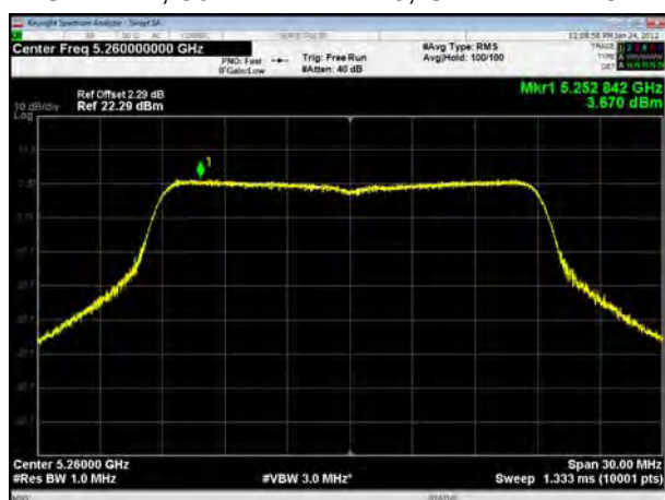
U-NII-2A, 802.11ac VHT20, Channel No.: 60
