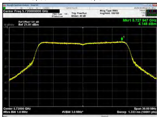
U-NII-2C, 802.11ac VHT40, Channel No.: 102
