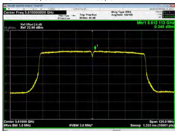
U-NII-2C, 802.11ac VHT80, Channel No.: 138
