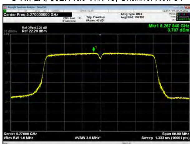
U-NII-2A, 802.11ac VHT40, Channel No.: 62
