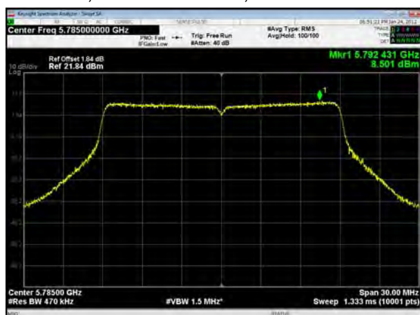
U-NII-3, 802.11ac VHT20, Channel No.: 157
