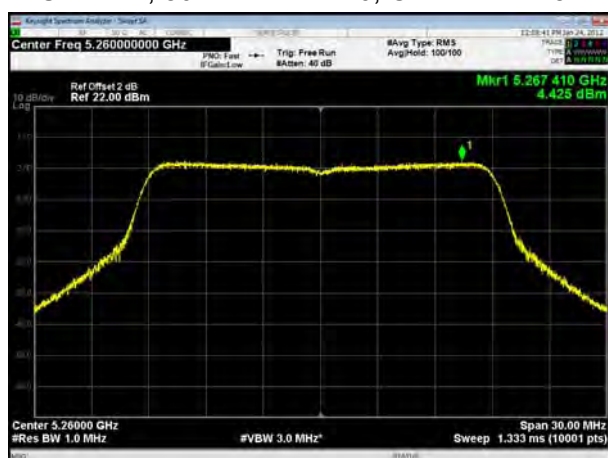
U-NII-2A, 802.11ac VHT20, Channel No.: 60
