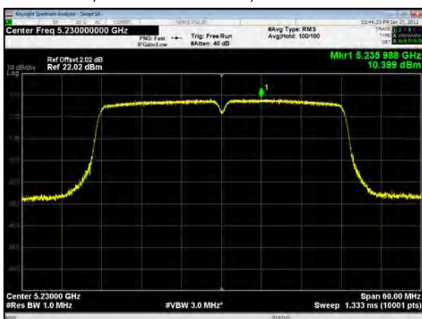
U-NII-1, 802.11ac VHT40, Channel No.: 46
