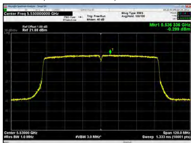
U-NII-2C, 802.11ac VHT80, Channel No.: 106
