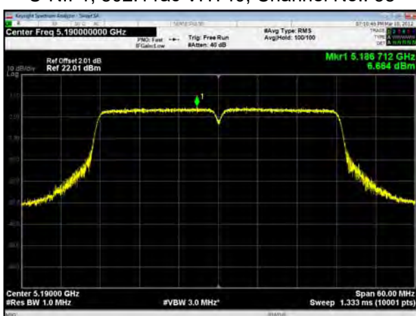
U-NII-1, 802.11ac VHT40, Channel No.: 46
