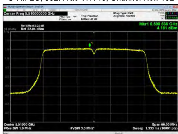
U-NII-2C, 802.11ac VHT40, Channel No.: 110
