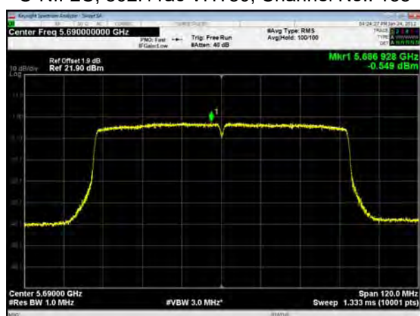
U-NII-2C, 802.11ac VHT160, Channel No.: 114
