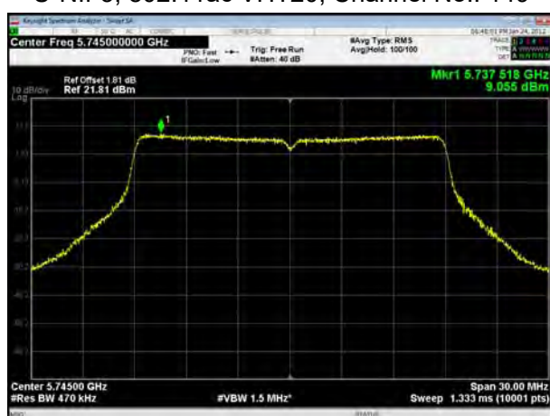
U-NII-3, 802.11ac VHT20, Channel No.: 157
