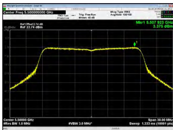
U-NII-2C, 802.11ac VHT20, Channel No.: 120
