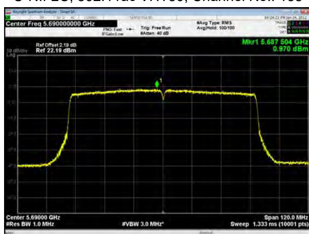
U-NII-2C, 802.11ac VHT160, Channel No.: 114
