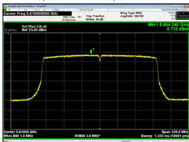
U-NII-2C, 802.11ac VHT80, Channel No.: 138
