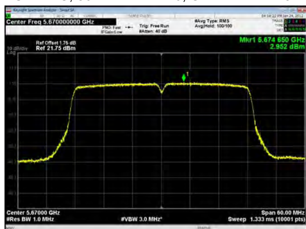
U-NII-2C, 802.11ac VHT40, Channel No.: 142
