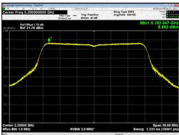
U-NII-1, 802.11ac VHT20, Channel No.: 40
