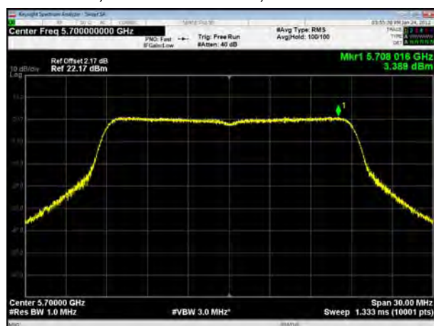
U-NII-2C, 802.11ac VHT20, Channel No.: 140
