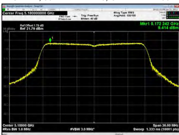
U-NII-1, 802.11ac VHT20, Channel No.: 40
