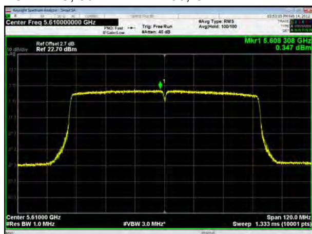
U-NII-2C, 802.11ac VHT80, Channel No.: 138
