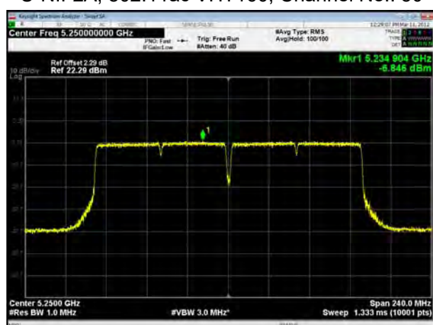
U-NII-2A, 802.11ac VHT160, Channel No.: 50
