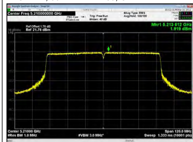
U-NII-1, 802.11ac VHT80, Channel No.: 42
