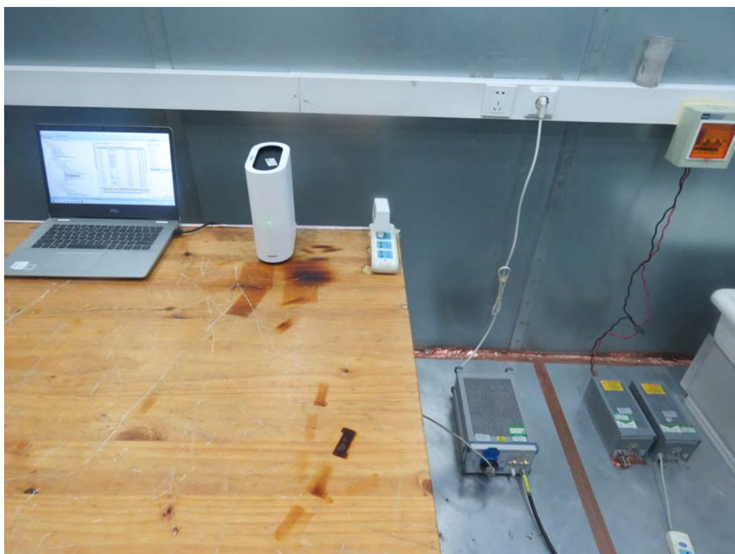
Picture 2 Conducted Emission Test Setup
