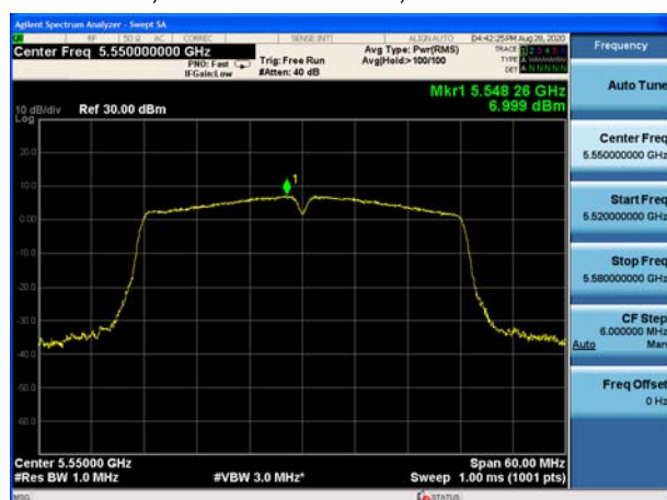
U-NII-2C, 802.11ac VHT40, Channel No.: 110
