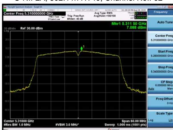
U-NII-2A, 802.11ac VHT40, Channel No.: 54
