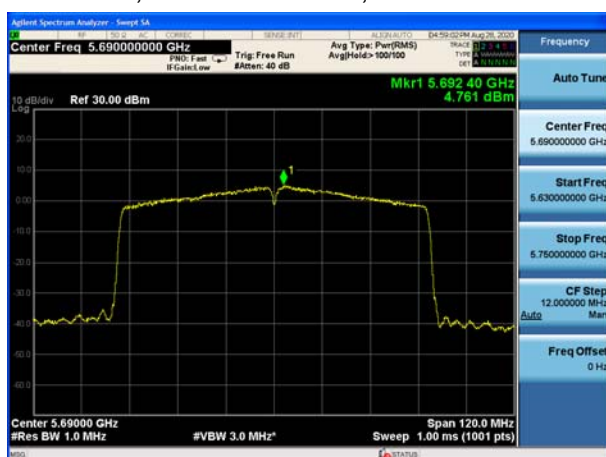
U-NII-2C, 802.11ac VHT80, Channel No.: 138
