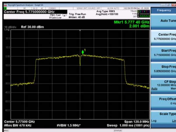
U-NII-3, 802.11ac VHT80, Channel No.: 155
