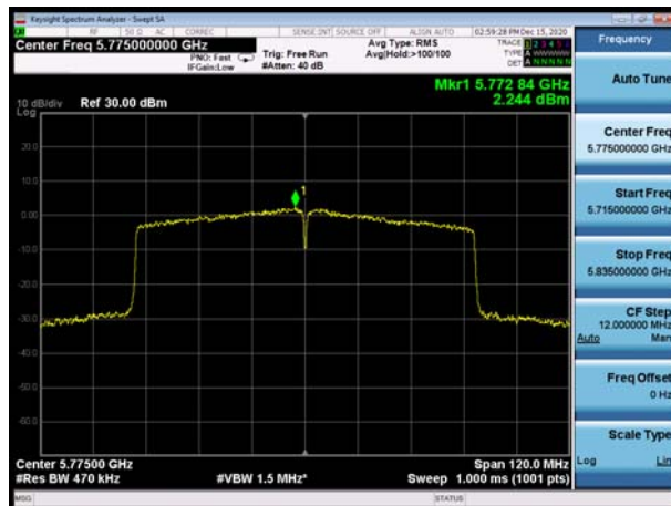
U-NII-3, 802.11ac VHT80, Channel No.: 155
