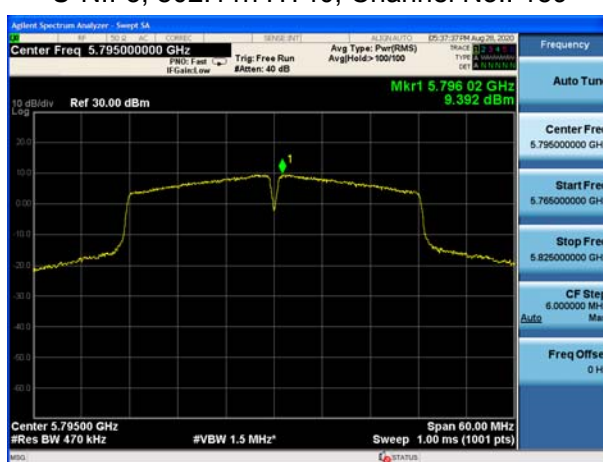
U-NII-3, 802.11ac VHT20, Channel No.: 149
