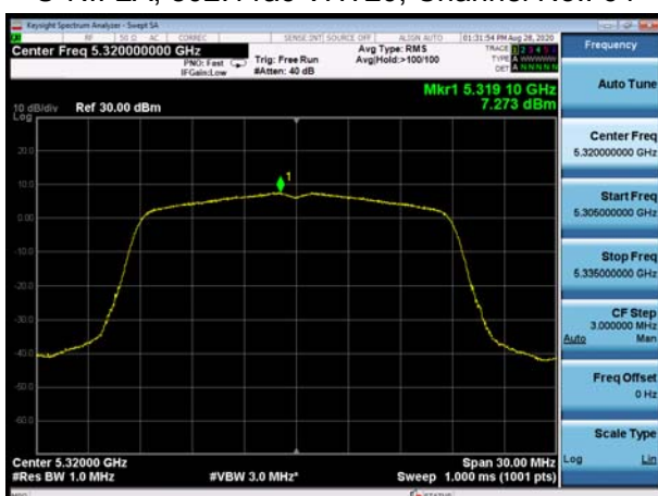
U-NII-2A, 802.11ac VHT20, Channel No.: 64
