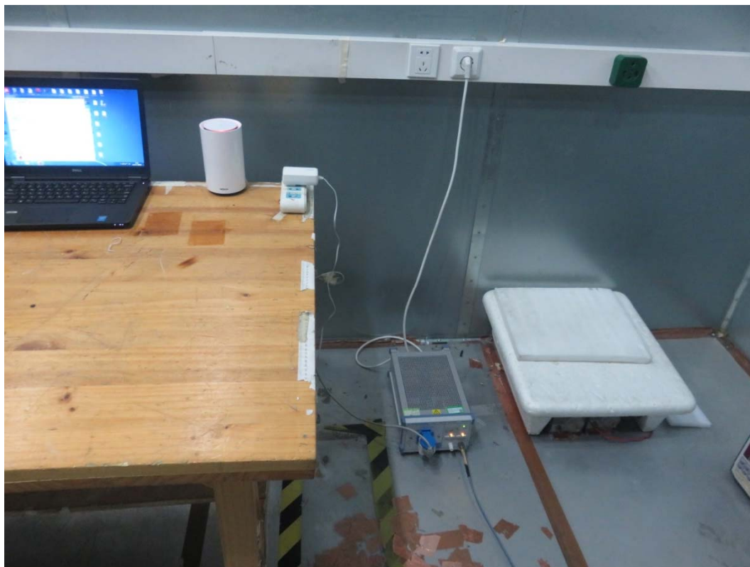
Picture 3 Conducted Emission Test Setup
