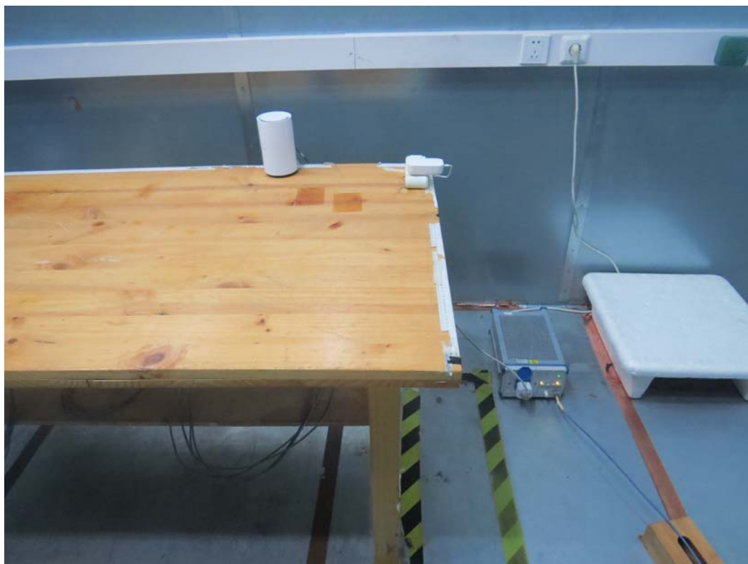
Picture 3 Conducted Emission Test Setup
