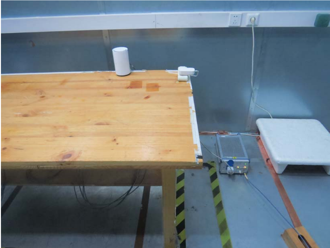
Picture 3 Conducted Emission Test Setup
