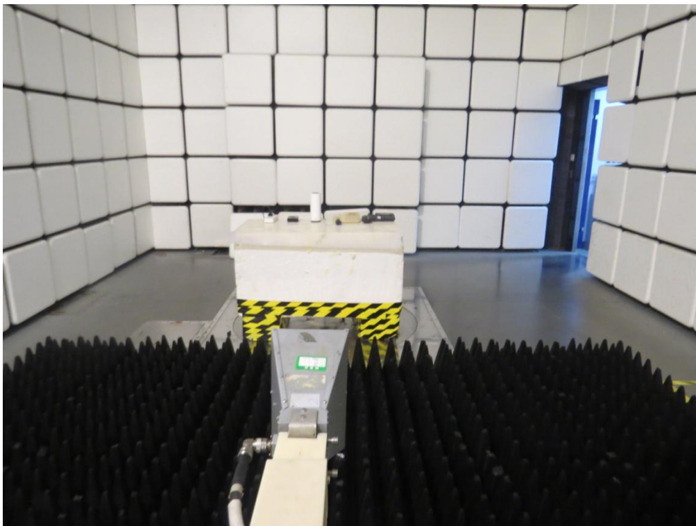
Picture 1 Radiated Emission Test Setup
