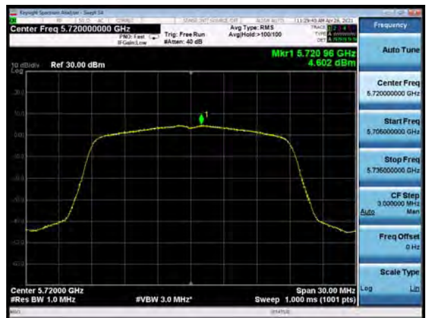
U-NII-2C, 802.11ac VHT20, Channel No.: 144
