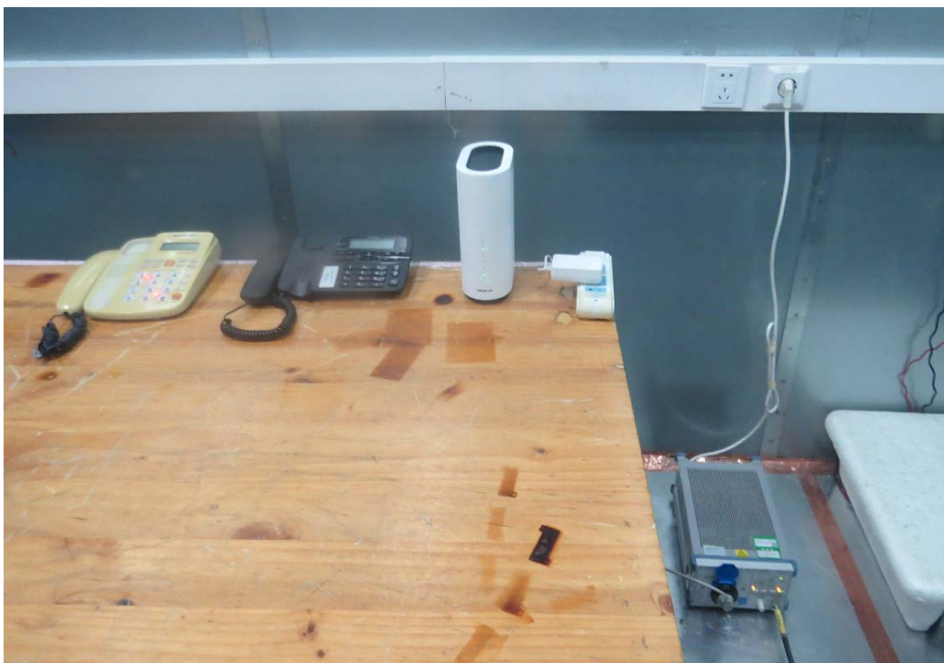
Picture 2 Conducted Emission Test Setup
