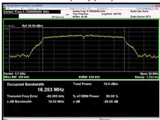
U-NII-2C, 802.11a Carrier frequency (MHz): 5700
