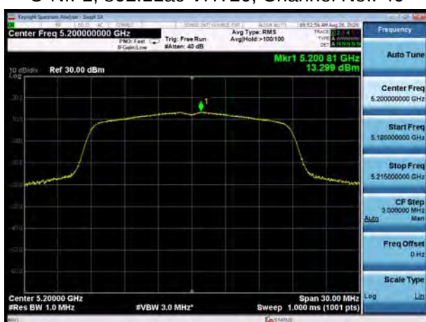
U-NII-1, 802.11ac VHT20, Channel No.: 48
