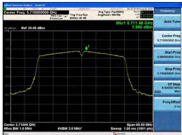
U-NII-2C, 802.11ac VHT40, Channel No.: 102
