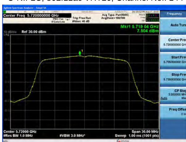
U-NII-2C, 802.11ac VHT80, Channel No.: 106
