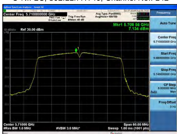
U-NII-2C, 802.11ac VHT40, Channel No.: 102
