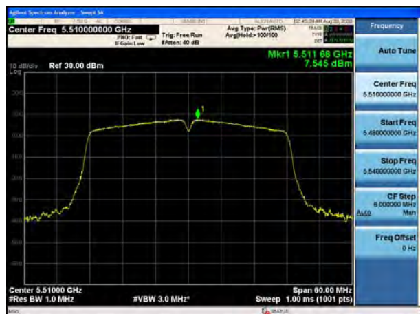
U-NII-2C, 802.11ac VHT40, Channel No.: 110
