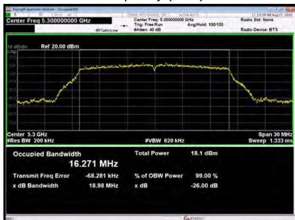
U-NII-2A, 802.11a Carrier frequency (MHz): 5320
