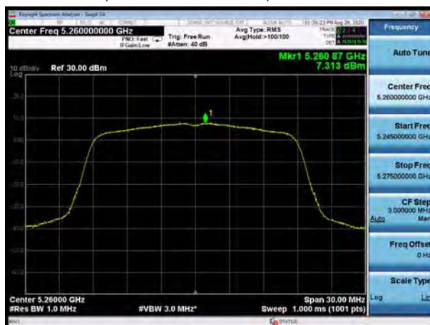
U-NII-2A, 802.11ac VHT20, Channel No.: 60
