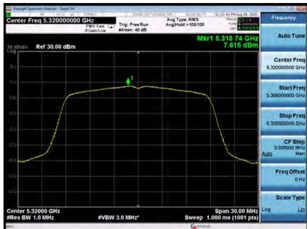
U-NII-2A, 802.11ac VHT20, Channel No.: 64
