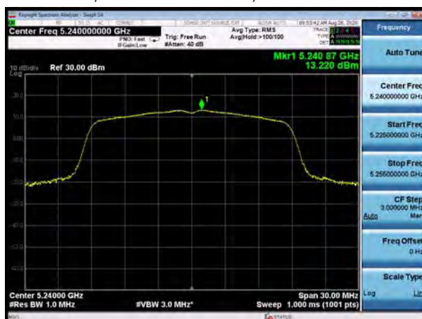
U-NII-1, 802.11ac VHT20, Channel No.: 48
