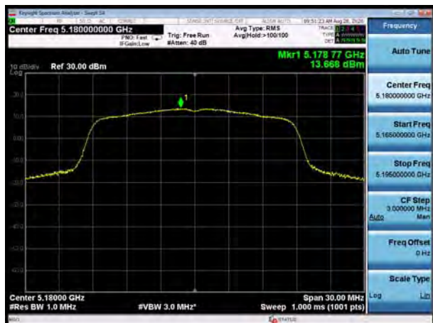
U-NII-1, 802.11ac VHT20, Channel No.: 40
