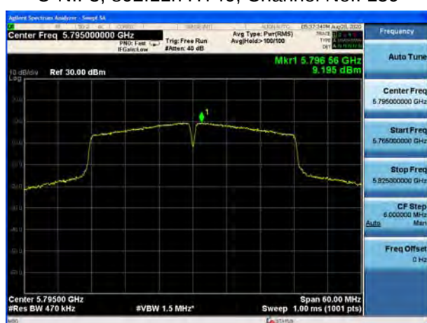
U-NII-3, 802.11ac VHT40, Channel No.: 151
