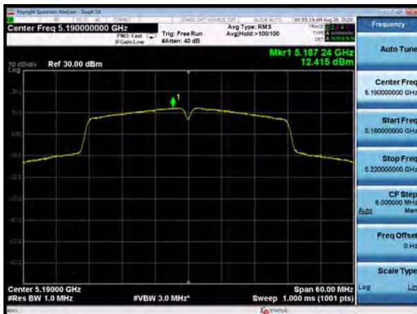
U-NII-1, 802.11ac VHT40, Channel No.: 38
