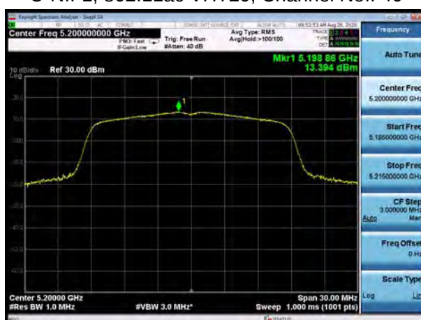
U-NII-1, 802.11ac VHT20, Channel No.: 48
