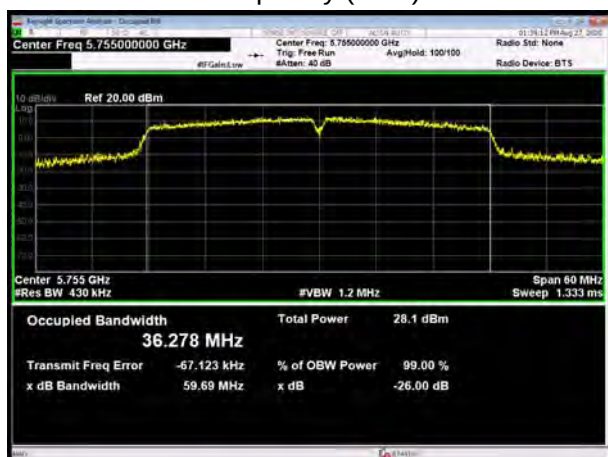
U-NII-3, 802.11n HT40 Carrier frequency (MHz): 5795
