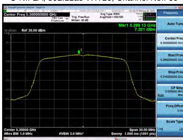
U-NII-2A, 802.11ac VHT20, Channel No.: 64
