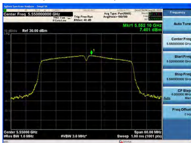
U-NII-2C, 802.11ac VHT40, Channel No.: 134
