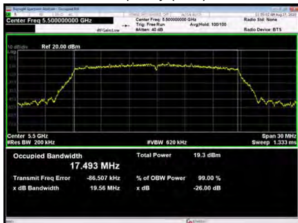
U-NII-2C, 802.11n HT20 Carrier frequency (MHz): 5580
