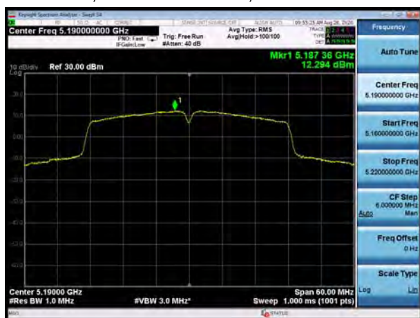
U-NII-1, 802.11ac VHT40, Channel No.: 38
