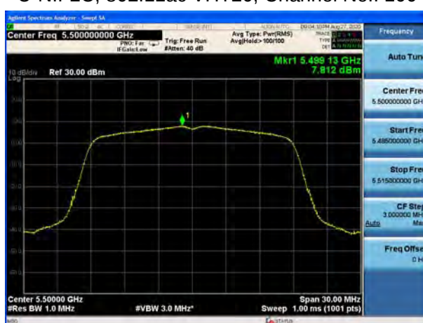
U-NII-2C, 802.11ac VHT20, Channel No.: 116
