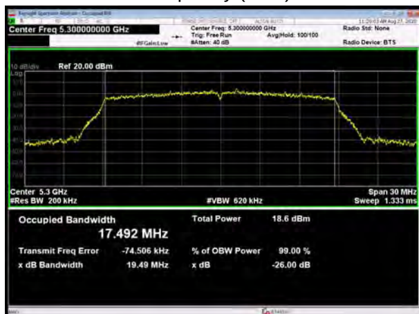
U-NII-2A, 802.11n HT20 Carrier frequency (MHz): 5320
