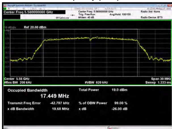
U-NII-2C, 802.11n HT20 Carrier frequency (MHz): 5700
