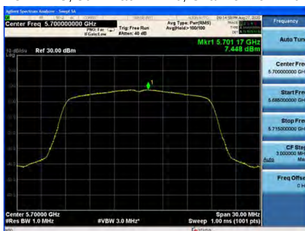
U-NII-2C, 802.11ac VHT20, Channel No.: 144
