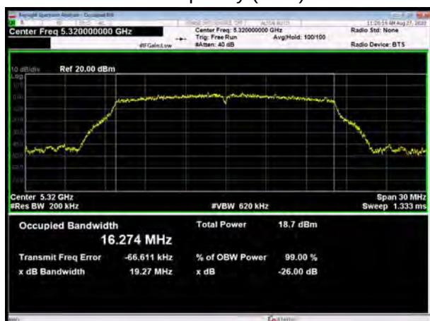
U-NII-2A, 802.11a Carrier frequency (MHz): 5320
