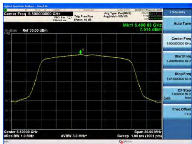
U-NII-2C, 802.11ac VHT20, Channel No.: 116
