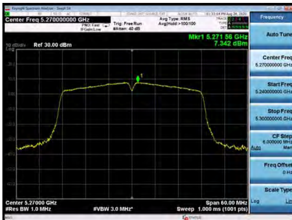
U-NII-2A, 802.11ac VHT40, Channel No.: 54
