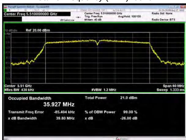
U-NII-2C, 802.11n HT40 Carrier frequency (MHz): 5550
