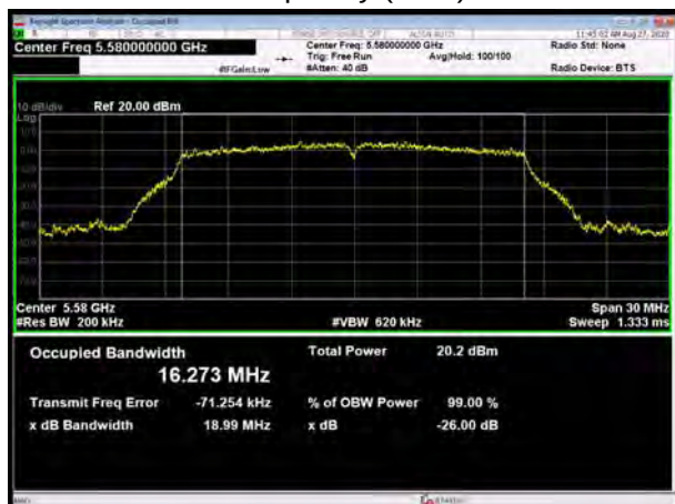
U-NII-2C, 802.11a Carrier frequency (MHz): 5700
