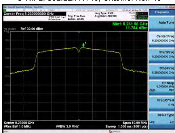
U-NII-1, 802.11ac VHT40, Channel No.: 38
