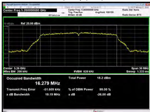
U-NII-2A, 802.11a Carrier frequency (MHz): 5300
