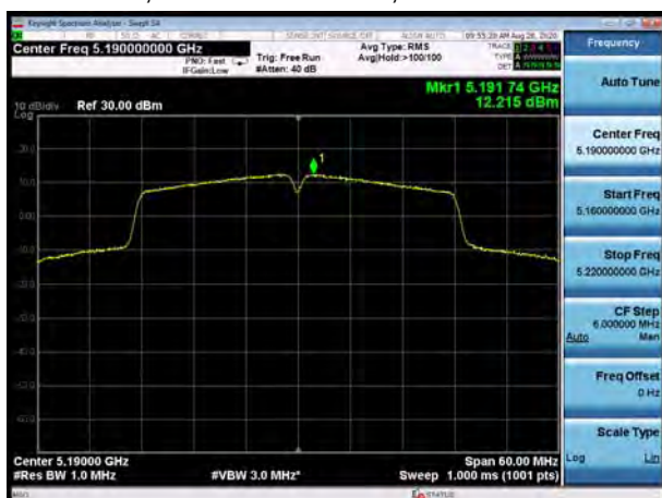
U-NII-1, 802.11ac VHT40, Channel No.: 38
