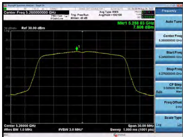
U-NII-2A, 802.11ac VHT20, Channel No.: 60
