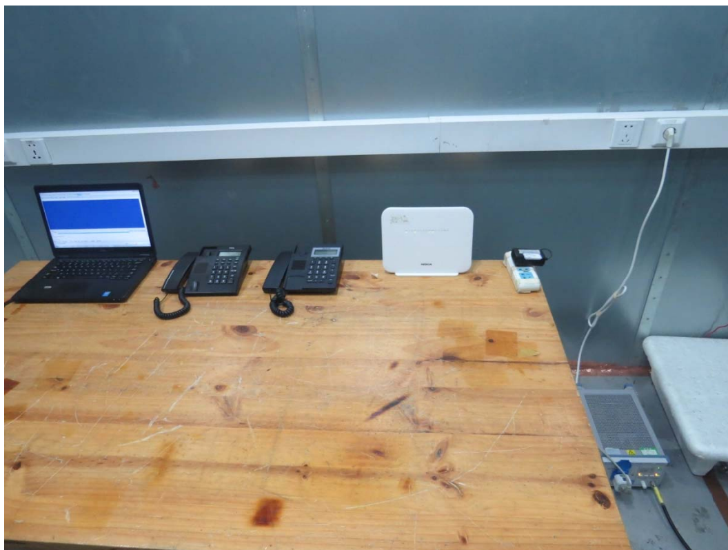
Picture 2 Conducted Emission Test Setup
