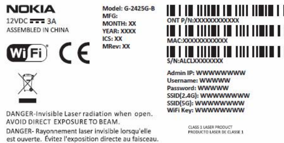
Figure 3-2 Sample laser product label showing CDRH 21 CFR compliance
