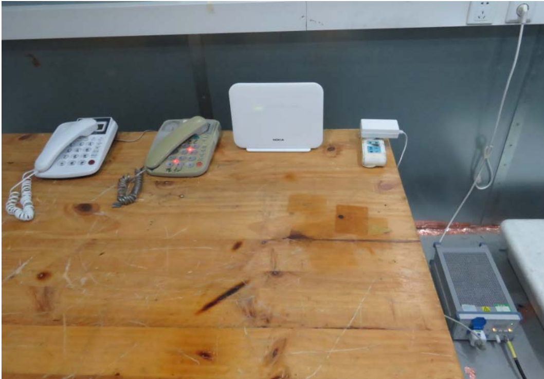
Picture 2 Conducted Emission Test Setup
