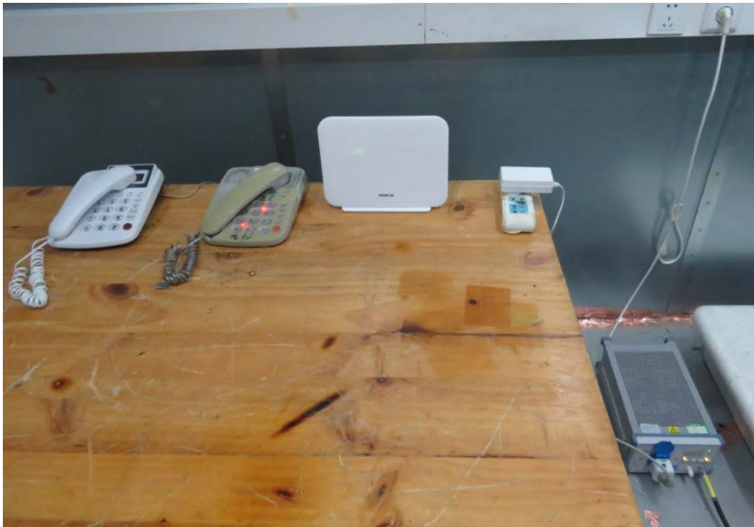
Picture 2 Conducted Emission Test Setup
