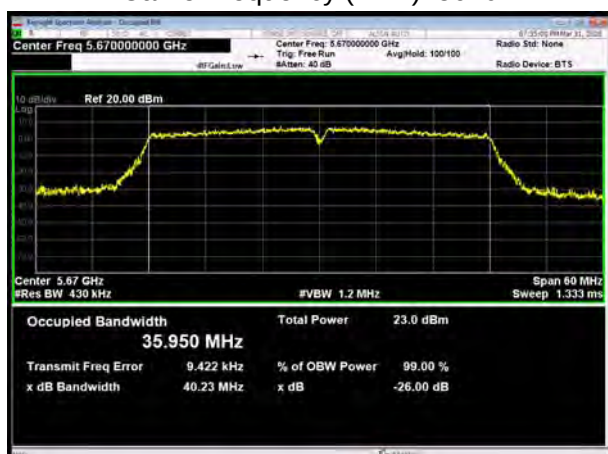
U-NII-2C, 802.11n HT40 Carrier frequency (MHz): 5710
