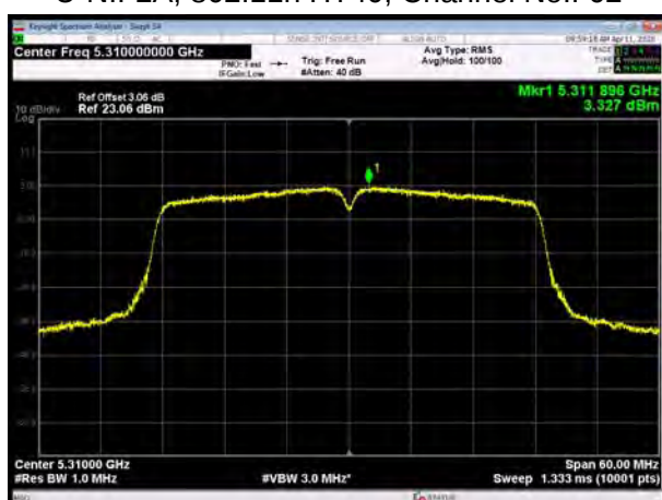
U-NII-2A, 802.11ac VHT40, Channel No.: 54
