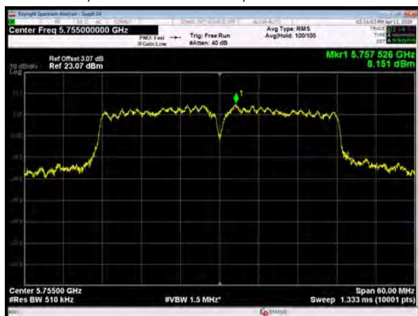
U-NII-3, 802.11ac VHT40, Channel No.: 151
