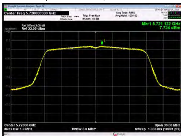
U-NII-2C, 802.11ac VHT20, Channel No.: 100
