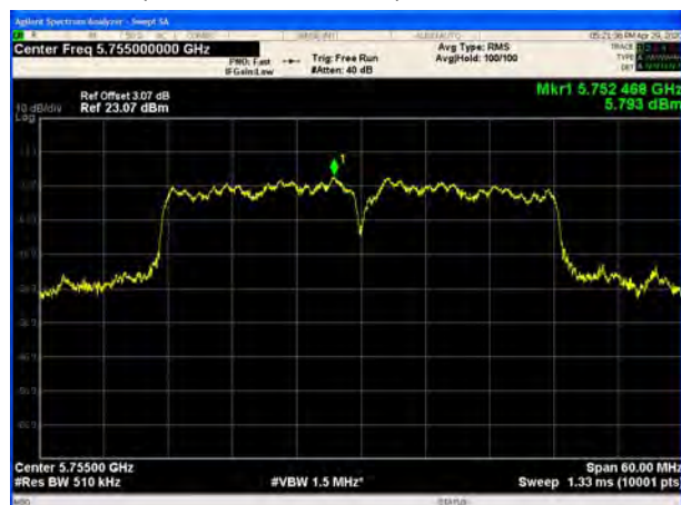
U-NII-3, 802.11ac VHT40, Channel No.: 151
