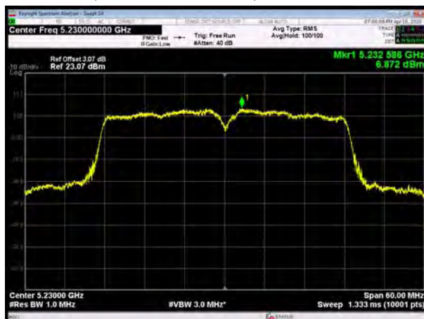
U-NII-1, 802.11ac VHT80, Channel No.: 42
