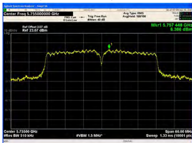
U-NII-3, 802.11ac VHT40, Channel No.: 151
