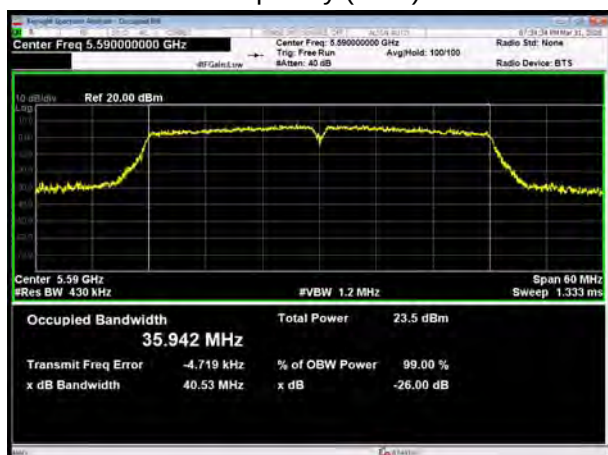
U-NII-2C, 802.11n HT40 Carrier frequency (MHz): 5670
