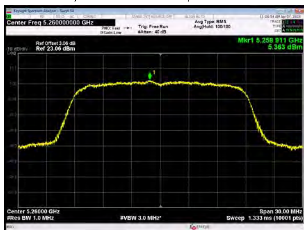
U-NII-2A, 802.11ac VHT20, Channel No.: 60
