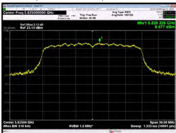
U-NII-3, 802.11ac VHT20, Channel No.: 165
