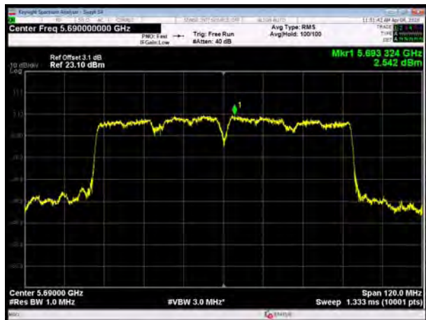
U-NII-2C, 802.11ac VHT80, Channel No.: 138
