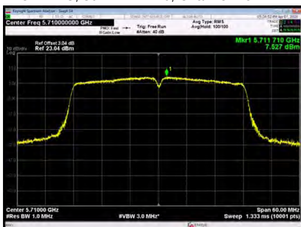
U-NII-2C, 802.11ac VHT40, Channel No.: 102
