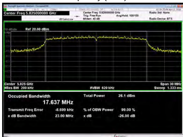
U-NII-3, 802.11n HT20 Carrier frequency (MHz): 5825
