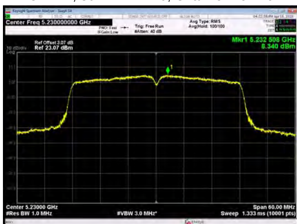
U-NII-1, 802.11ac VHT40, Channel No.: 38
