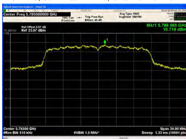
U-NII-3, 802.11ac VHT20, Channel No.: 165
