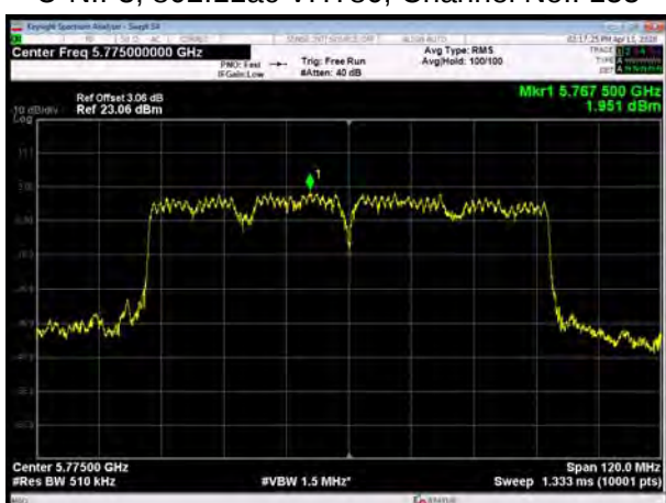
U-NII-3, 802.11ac VHT80, Channel No.: 155
