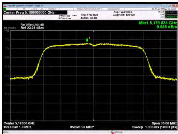
U-NII-1, 802.11ac VHT20, Channel No.: 40
