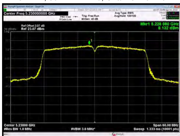
U-NII-1, 802.11ac VHT40, Channel No.: 38
