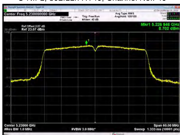
U-NII-1, 802.11ac VHT40, Channel No.: 38
