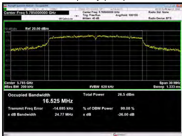
U-NII-3, 802.11a Carrier frequency (MHz): 5825
