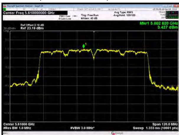
U-NII-2C, 802.11ac VHT80, Channel No.: 122
