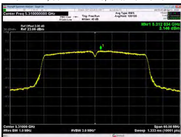
U-NII-2A, 802.11ac VHT40, Channel No.: 54
