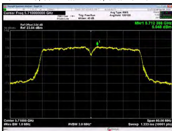
U-NII-2C, 802.11ac VHT80, Channel No.: 138
