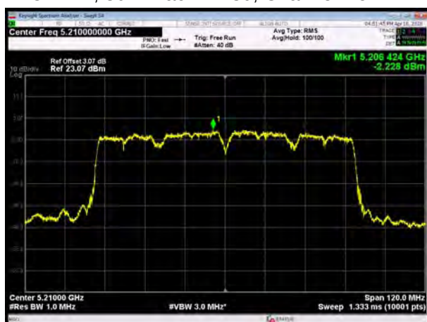
U-NII-1, 802.11ac VHT80, Channel No.: 42
