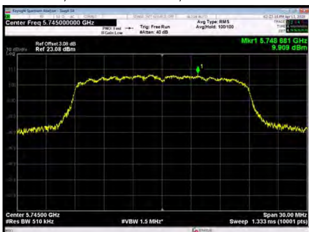
U-NII-3, 802.11ac VHT20, Channel No.: 157
