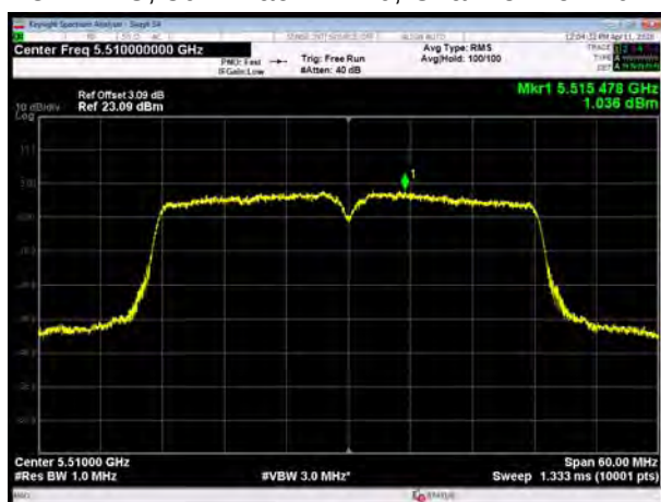
U-NII-2C, 802.11ac VHT40, Channel No.: 118
