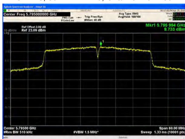
U-NII-3, 802.11ac VHT40, Channel No.: 151
