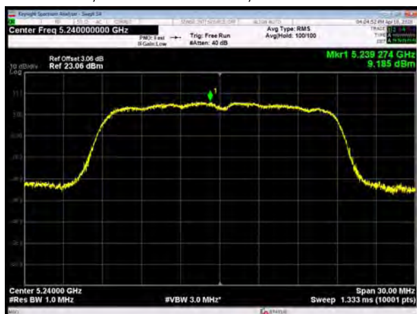
U-NII-1, 802.11ac VHT20, Channel No.: 48
