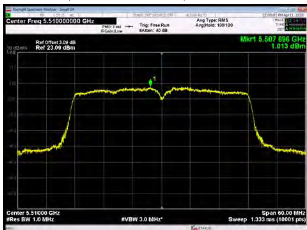
U-NII-2C, 802.11ac VHT40, Channel No.: 102
