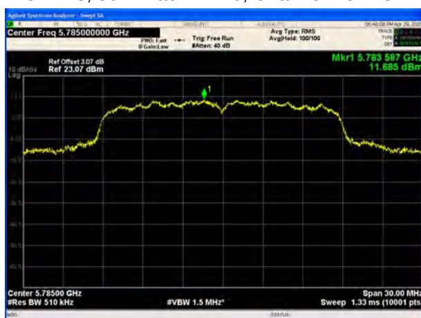
U-NII-3, 802.11ac VHT20, Channel No.: 165
