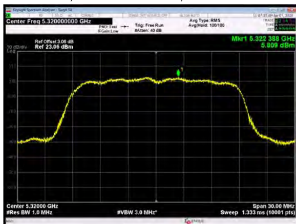
U-NII-2A, 802.11ac VHT20, Channel No.: 64
