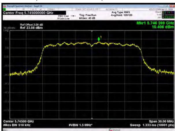
U-NII-3, 802.11ac VHT20, Channel No.: 157
