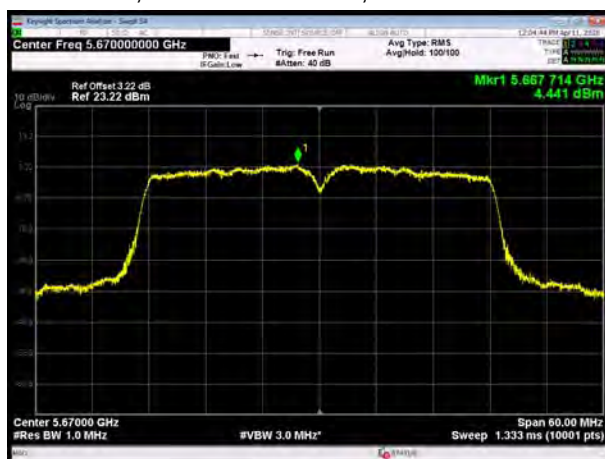
U-NII-2C, 802.11ac VHT40, Channel No.: 142
