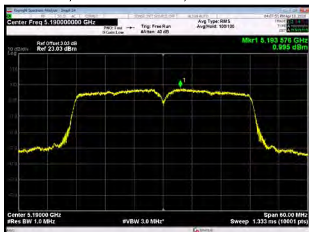
U-NII-1, 802.11ac VHT40, Channel No.: 38
