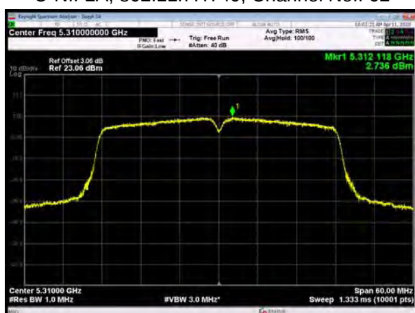
U-NII-2A, 802.11ac VHT40, Channel No.: 54
