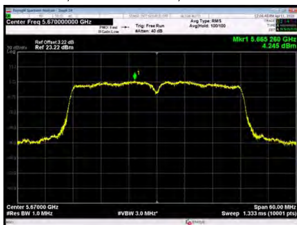
U-NII-2C, 802.11ac VHT40, Channel No.: 142
