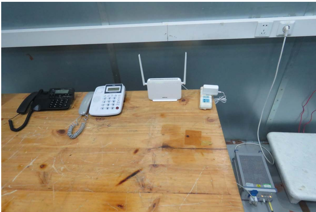
Picture 2 Conducted Emission Test Setup
