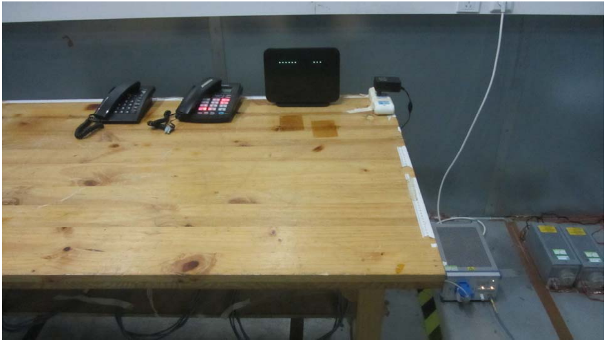
Picture 3 Conducted Emission Test Setup
