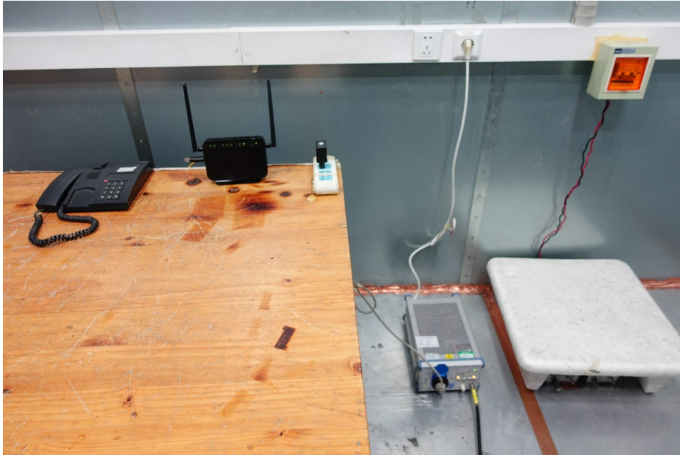
Picture 2: Conducted Emissions Test Setup
