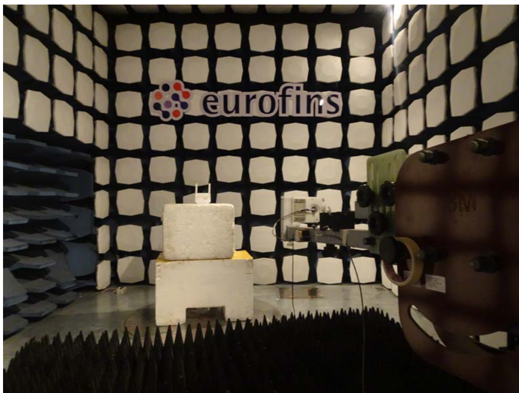
Picture 1 Radiated Emission Test Setup
