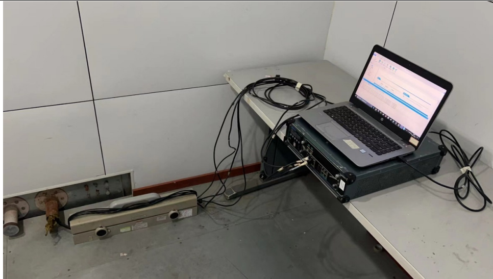
Auxiliary test equipment Picture 1: Radiated Emission Test Setup
