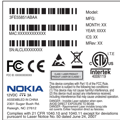
Figure 4-2 Sample laser product label showing CDRH 21 CFR compliance
