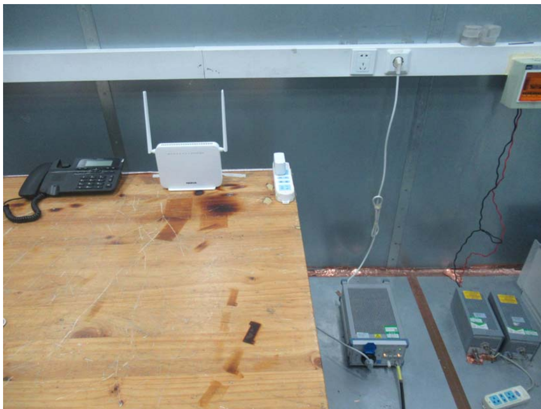
Picture 2 Conducted Emission Test Setup
