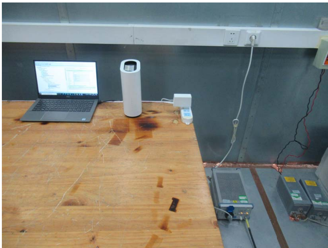
Picture 2 Conducted Emission Test Setup
