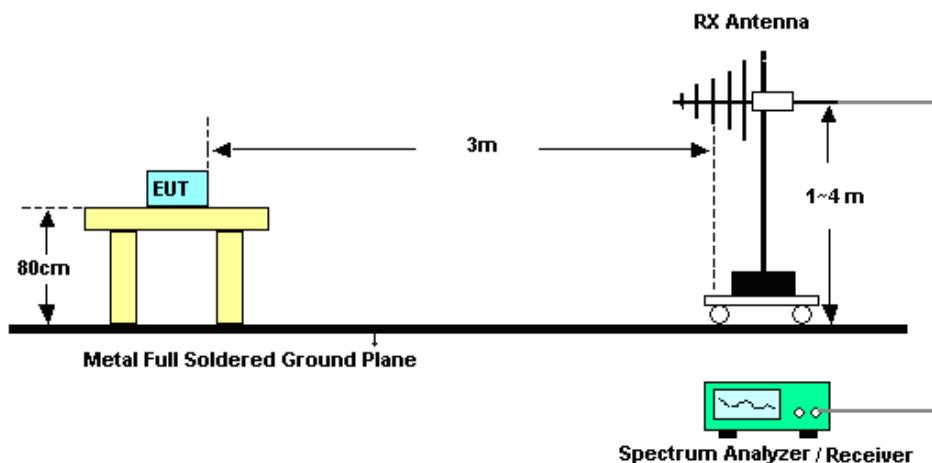
**For radiated emissions above 1GHz**
