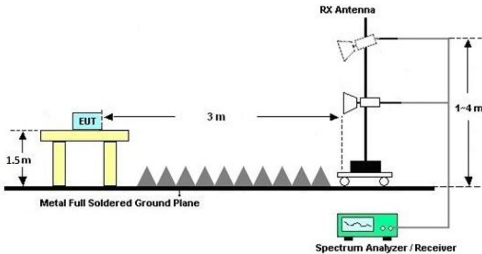
**3.5.5 Test Results of Radiated Spurious Emissions (9 kHz ~ 30 MHz)**
