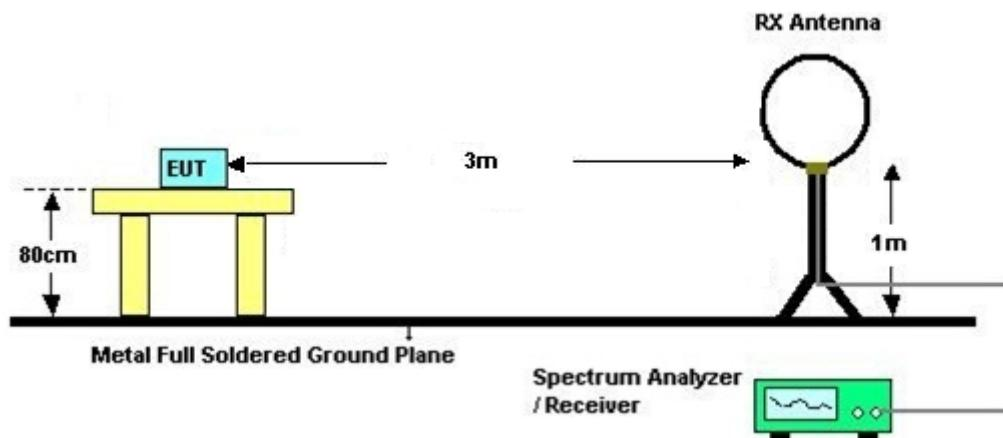
For radiated emissions from 30MHz to 1GHz
