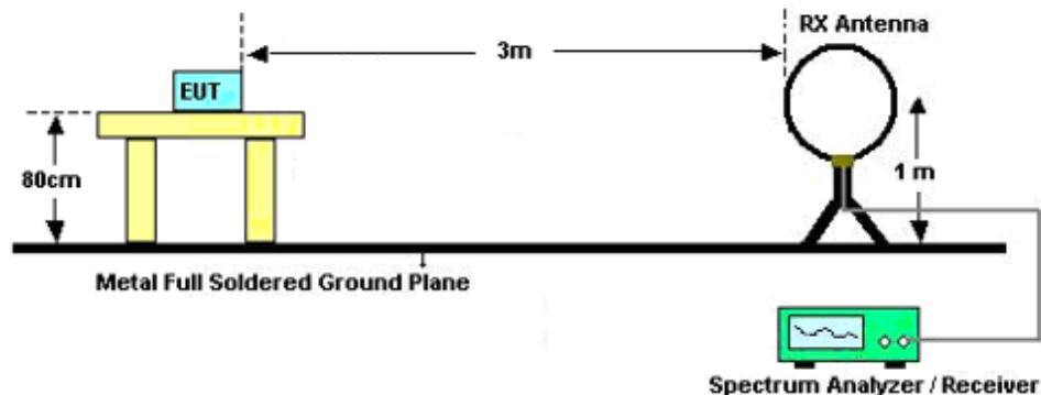
For radiated emissions from 30MHz to 1GHz
