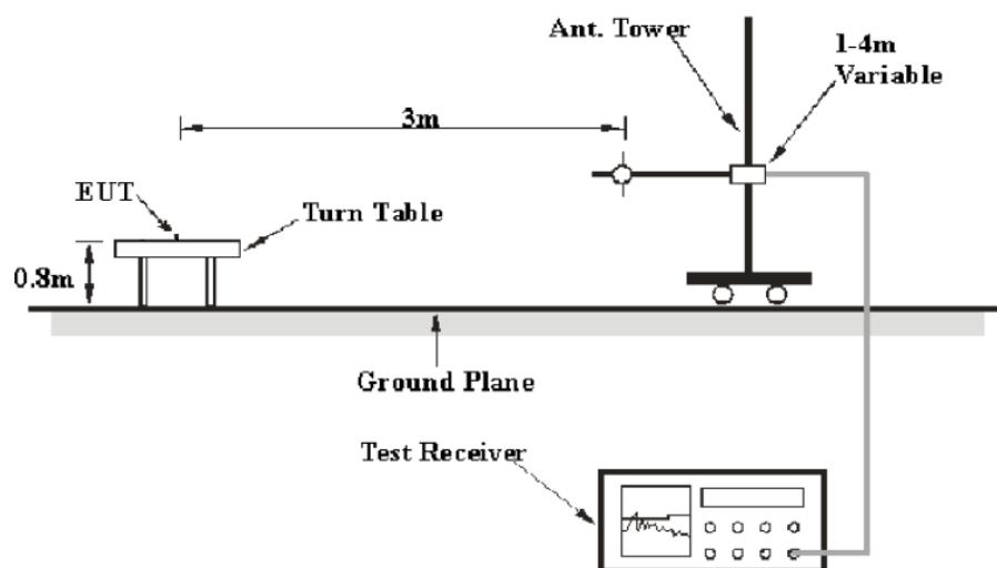
The radiated emission tests were performed in the 3-meter chamber a test site, using the setup accordance with the ANSI C63.10. The specification used was the FCC 15.205, 15.209 and FCC 15.255 limits.
