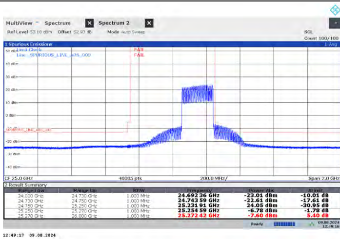
n258-b 200MHz-64QAM- High -H-1RB131
