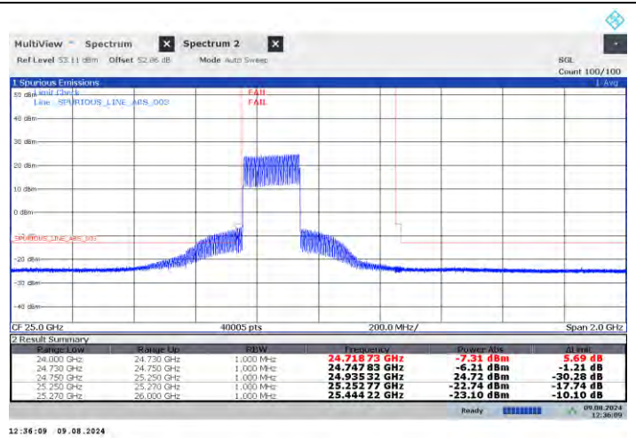
n258-b 200MHz-64QAM -Low -V-1RB0
