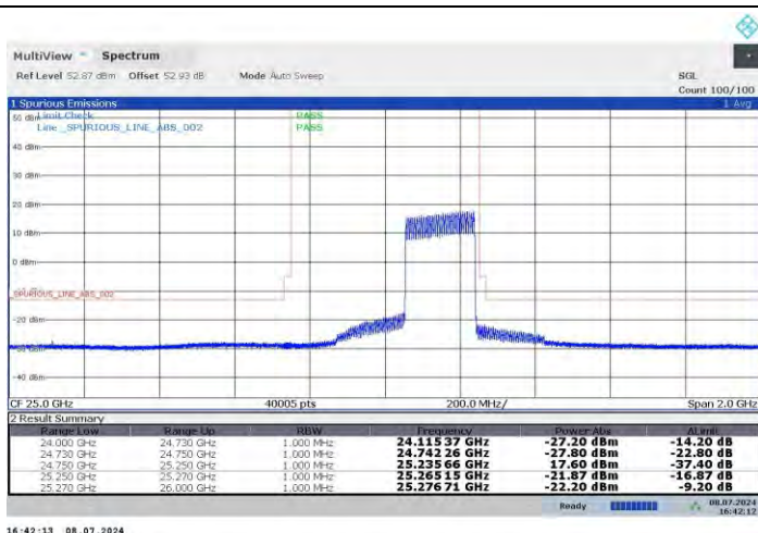
n258-b 200MHz-64QAM - High -H-128RB0
