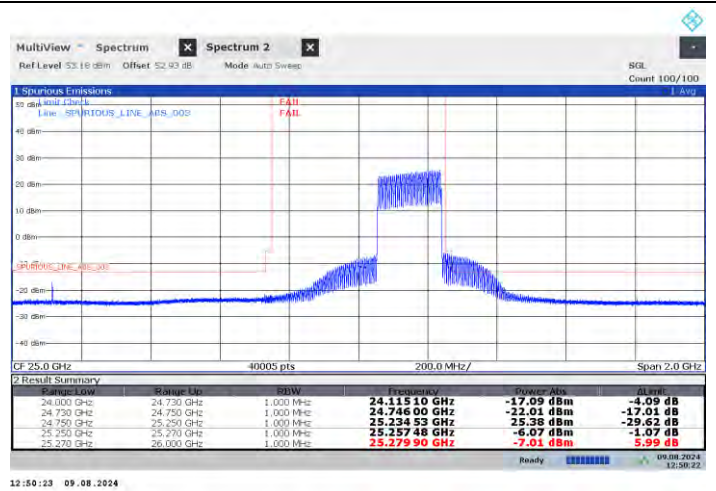
n258-b 200MHz-64QAM - High -V-1RB131
