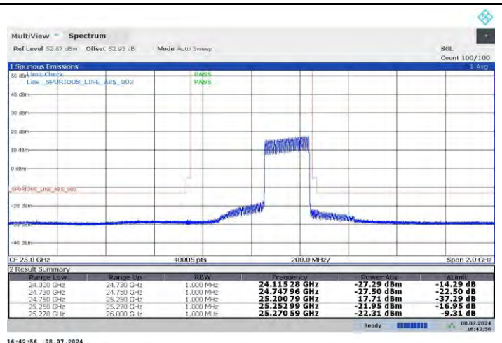
n258-b 200MHz -64QAM - High -V-128RB0
