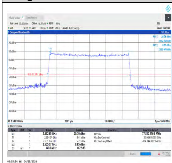
1-N41-30-80-M-3-DFT-16QAM-Out_ Full-21 6@0-Ant1-77.312-80.800-≤80-PASS
