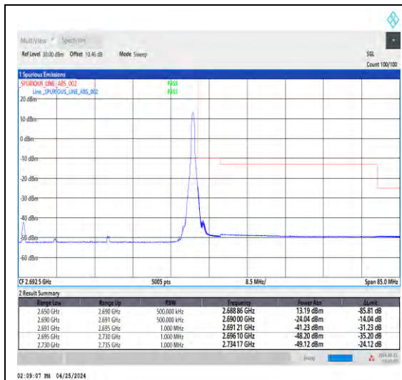
1-N41-30-40-H-5-CP-QPSK-Edge_1RB_Righ t-1@105-Ant1-1--PASS-see graph
