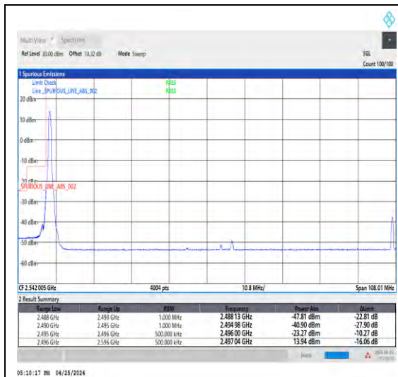
1-N41-30-100-L-1-DFT-PI2BPSK-Edge_1RB _Left-1@0-Ant1-1--PASS-see graph
