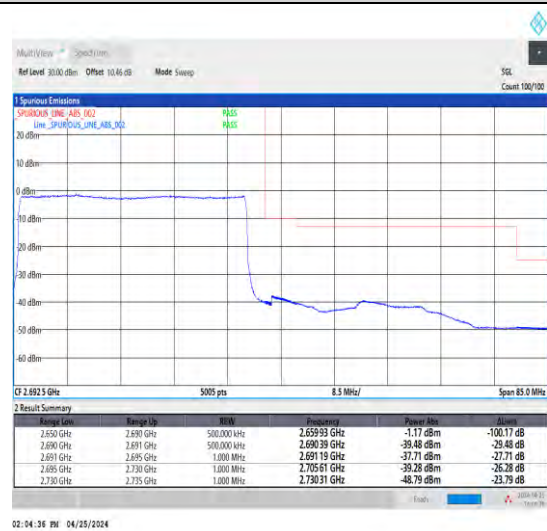
1-N41-30-40-H-3-DFT-PI2BPSK-Outer_Full-1 00@0-Ant1-1--PASS-see graph
