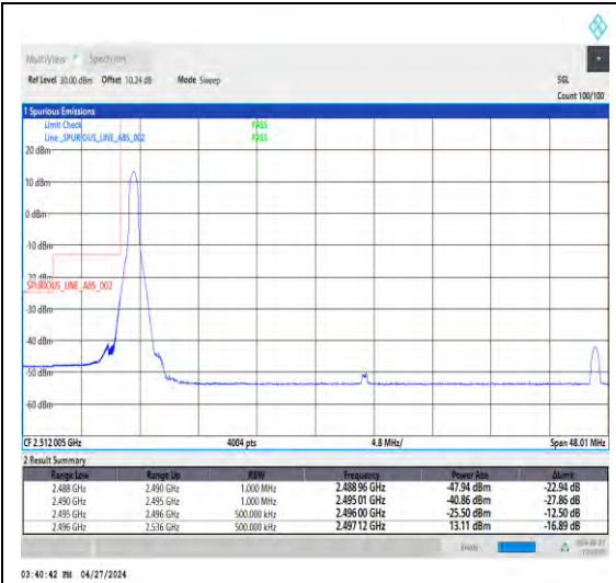
1-N41-30-40-L-1-DFT-PI2BPSK-Edge_1RB_ Left-1@0-Ant1-1--PASS-see graph
