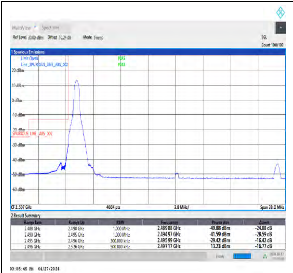
1-N41-30-30-L-1-DFT-PI2BPSK-Edge_1RB_ Left-1@0-Ant1-1--PASS-see graph
