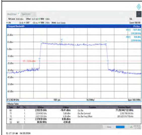
1-N41-30-80-M-1-DFT-QPSK-Out_ Full-216 @0-Ant1-77.292-80.960-≤80-PASS
