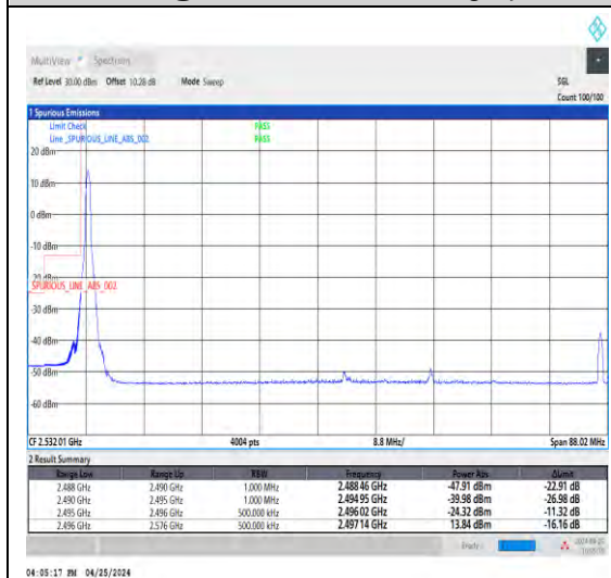
1-N41-30-80-L-4-CP-QPSK-Edge_1RB_Left- 1@0-Ant1-1--PASS-see graph
