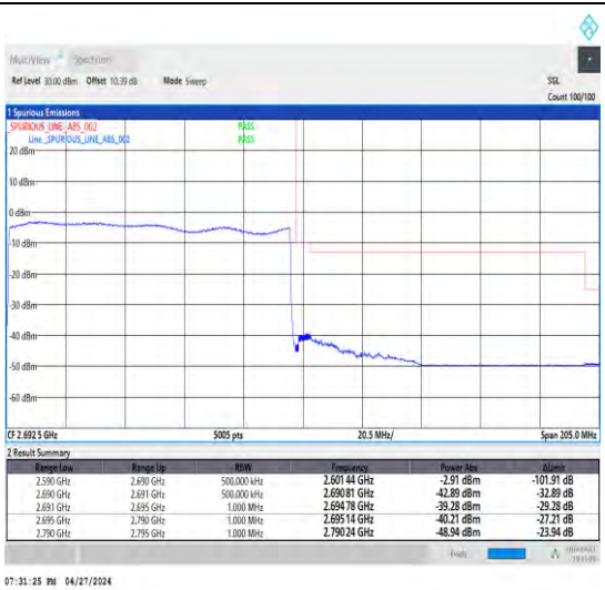
1-N41-30-100-H-3-DFT-PI2BPSK-Outer_Full- 270@0-Ant1-1--PASS-see graph
