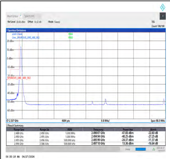
1-N41-30-90-L-1-DFT-PI2BPSK-Edge_1RB_ Left-1@0-Ant1-1--PASS-see graph
