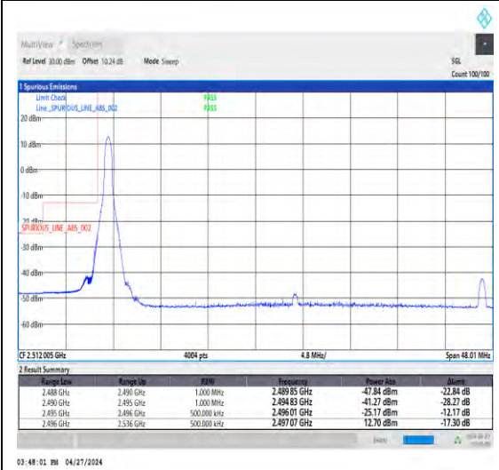
1-N41-30-40-L-4-CP-QPSK-Edge_1RB_Left- 1@0-Ant1-1--PASS-see graph
