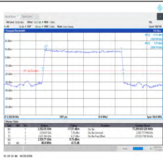
1-N41-30-80-M-2-DFT-PI2BPSK-Out_ Full- 216@0-Ant1-77.296-80.800-≤80-PASS
