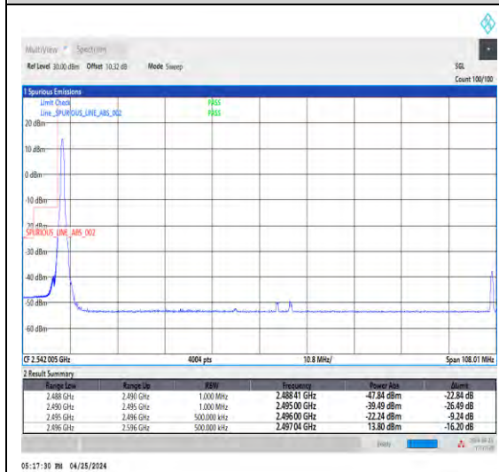
1-N41-30-100-L-4-CP-QPSK-Edge_1RB_Left -1@0-Ant1-1--PASS-see graph
