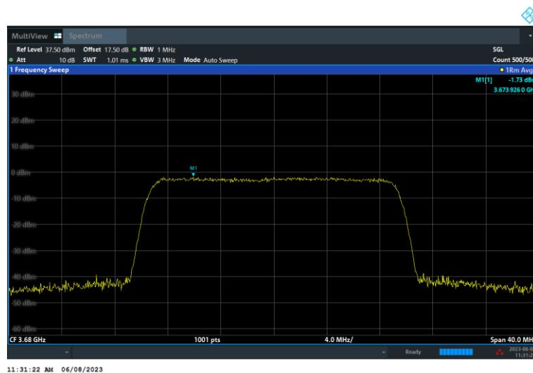
**SAS Granted MaxEIRP 24 [dBm/MHz]****UUT Center Frequency 3680 MHz, Bandwidth 20 MHz, MaxEIRP 22.68 [dBm/MHz]****TX 0**
