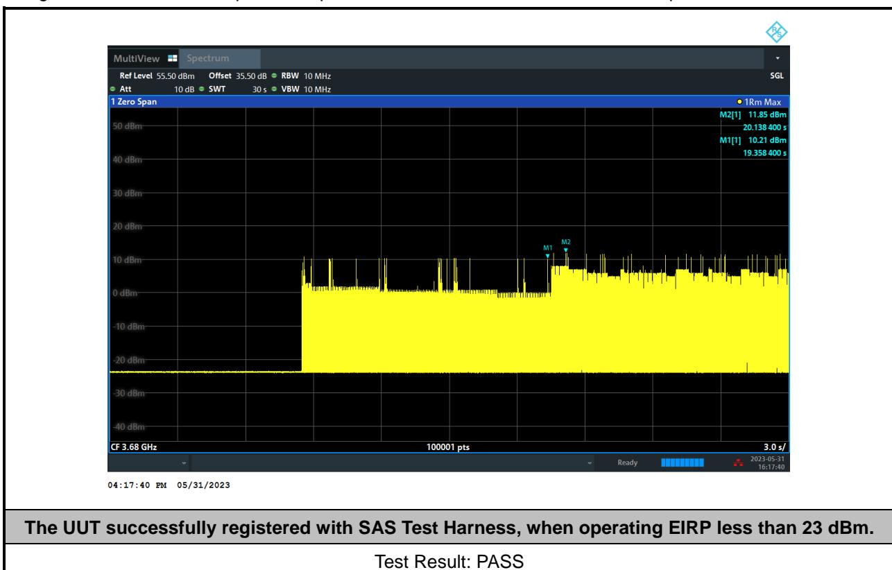
Note: The total offset 35.5 dB includes the antenna gain 18 dBi and cable path loss 17.5 dB.
