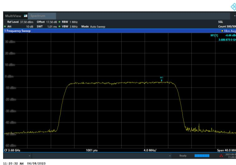
**SAS Granted MaxEIRP 37 [dBm/MHz]****UUT Center Frequency 3620 MHz, Bandwidth 40 MHz, MaxEIRP 24.27 [dBm/MHz]****TX 0**
