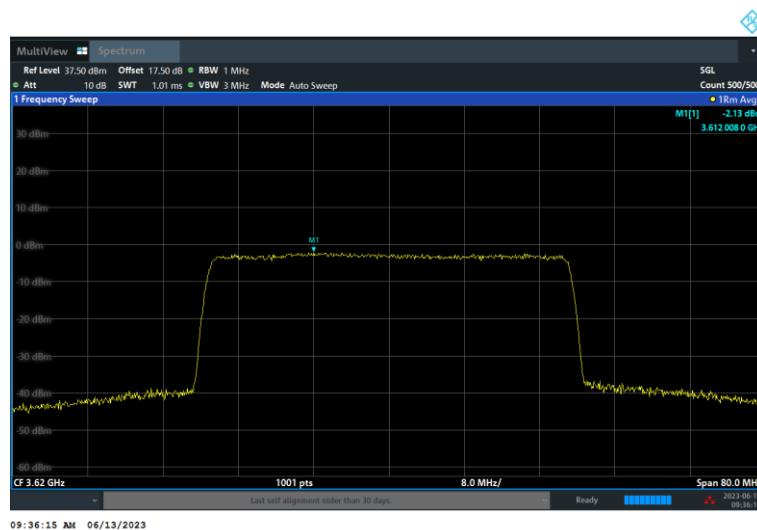
**SAS Granted MaxEIRP 26 [dBm/MHz]****UUT Center Frequency 3620 MHz, Bandwidth 40 MHz, MaxEIRP 23.07 [dBm/MHz]****TX 0**
