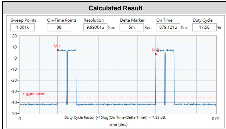
Note: The duty cycle value is 17.58%, add  $10\log(1/\text{duty cycle})$  to the measured power level to compute the average power during continuous transmission.
