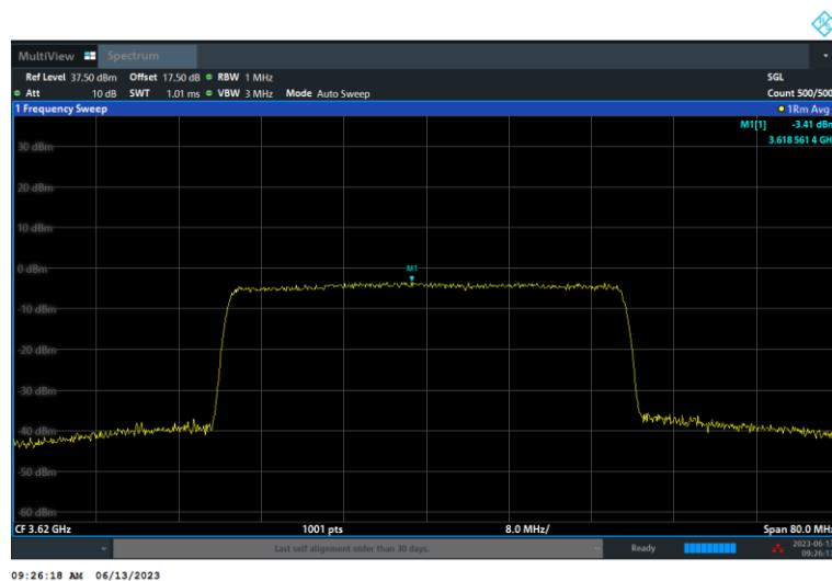
**SAS Granted MaxEIRP 23 [dBm/MHz]****UUT Center Frequency 3620 MHz, Bandwidth 40 MHz, MaxEIRP 21.2 [dBm/MHz]****TX 0**
