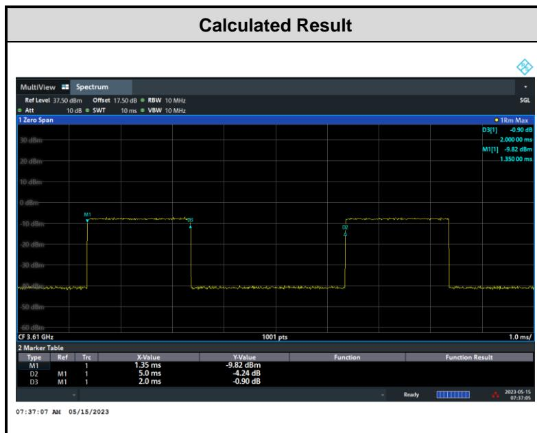
Note: The duty cycle value is 40%, add  $10\log(1/\text{duty cycle})$  to the measured power level to compute the average power during continuous transmission.
