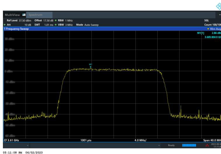
**SAS Granted MaxEIRP 24 [dBm/MHz]****UUT Center Frequency 3610 MHz, Bandwidth 20 MHz, MaxEIRP 23.29 [dBm/MHz]****TX 0**
