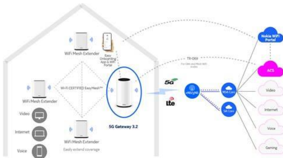
Figure 12 Nokia FastMile 5G Gateway 3.2 fixed wireless access end-to-end overview
