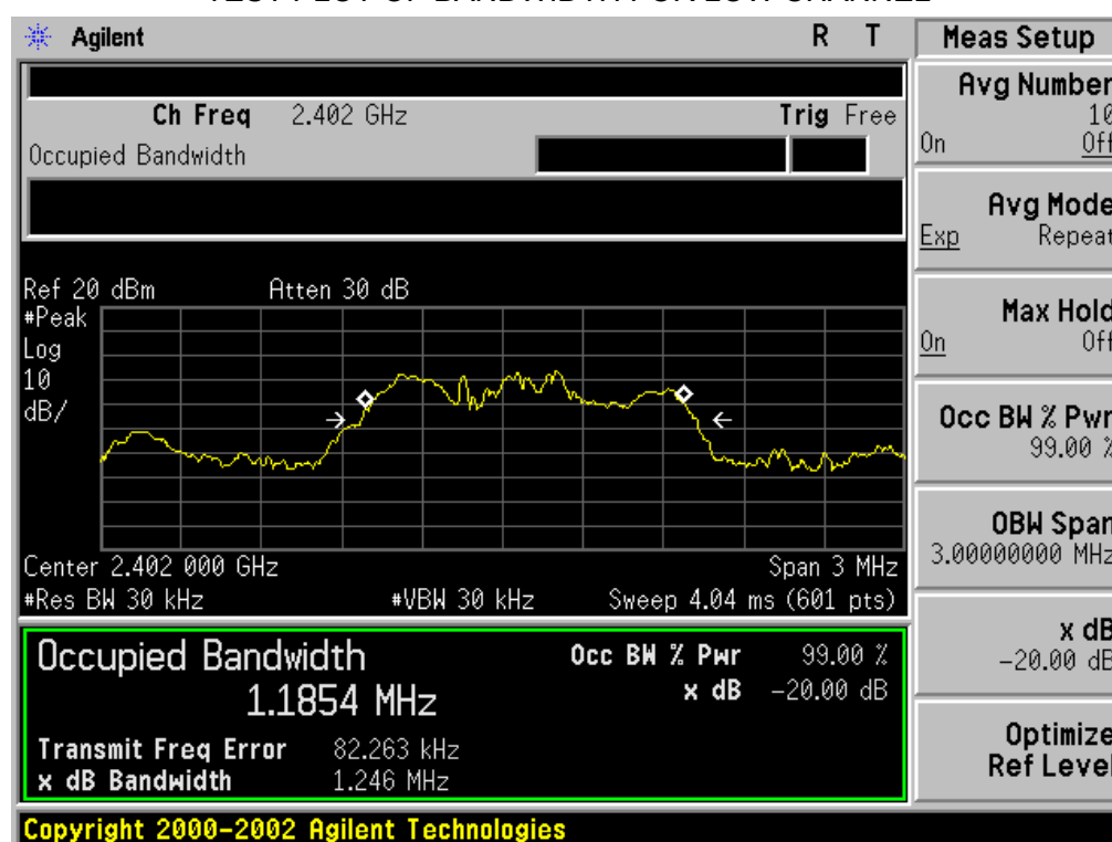
TEST PLOT OF BANDWIDTH FOR LOW CHANNEL
