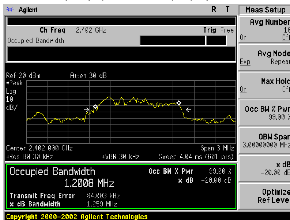
TEST PLOT OF BANDWIDTH FOR LOW CHANNEL
