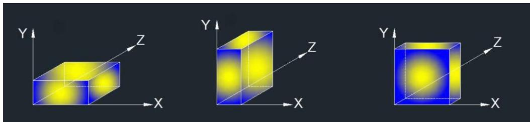
Note 1: For all radiated test, EUT in each of three orthogonal axis emissions had been tested, but only the worst case (Y axis) data recorded in the report.
