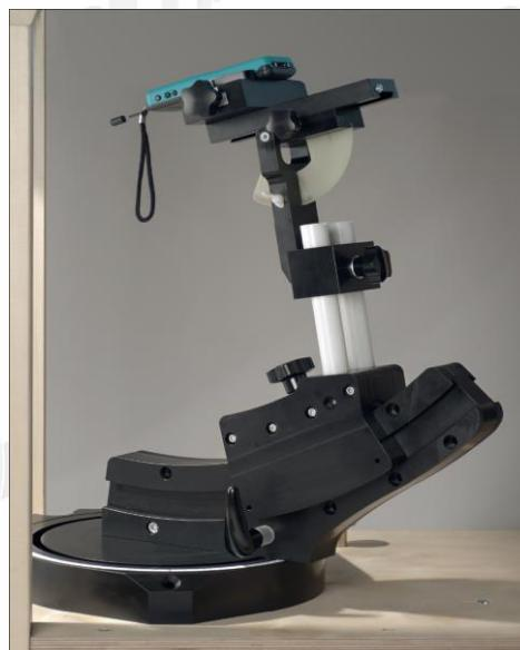
The DASY device holder is designed to cope with different positions given in the standard. It has two scales for the device rotation (with respect to the body axis) and the device inclination (with respect to the line between the ear reference points). The rotation centres for both scales are the ear reference point (ERP). Thus the device needs no repositioning when changing the angles.
