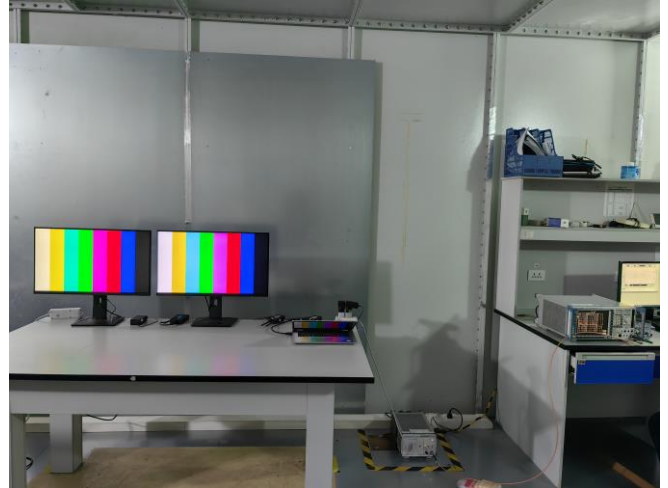
Conducted Emission on AC Mains
